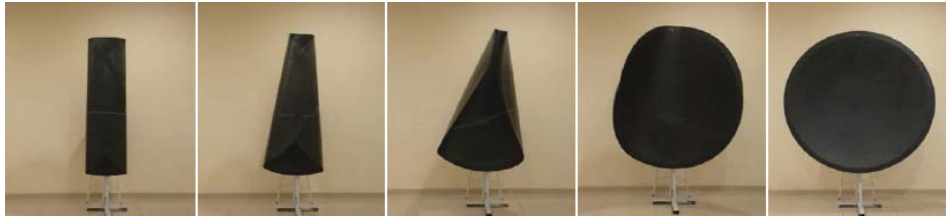
Figure 2.14: Deployment of the self-deployable shell reflector (duration: 1.4 s) [15]
