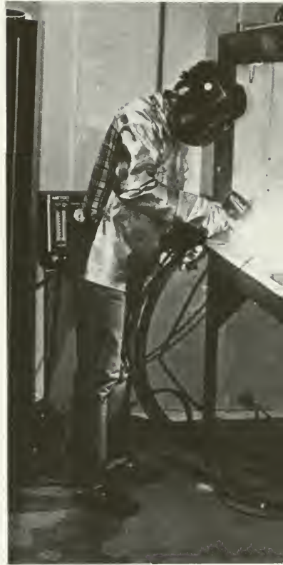
Graduate student Joe Grindley coats engine components with ceramic materials at the Plasma Spray Booth in the Ceramic Engineering Building (Photo by Eric Smith).
