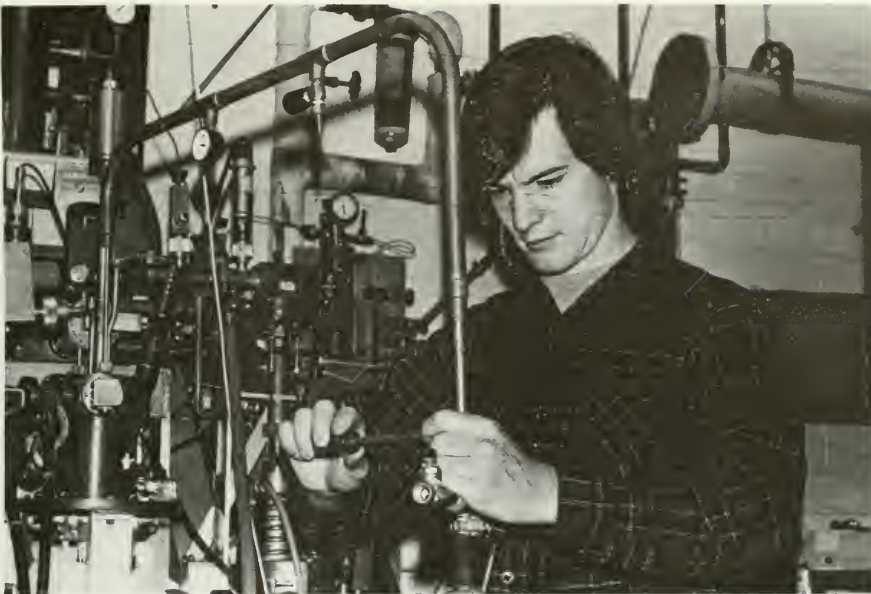
Mark Reeves, graduate student in physics, patiently fills a dewar flask with liquid helium in order to carry out low-temperature calorimetry experiments on superconducting materials (Photo by Dan Powers).
