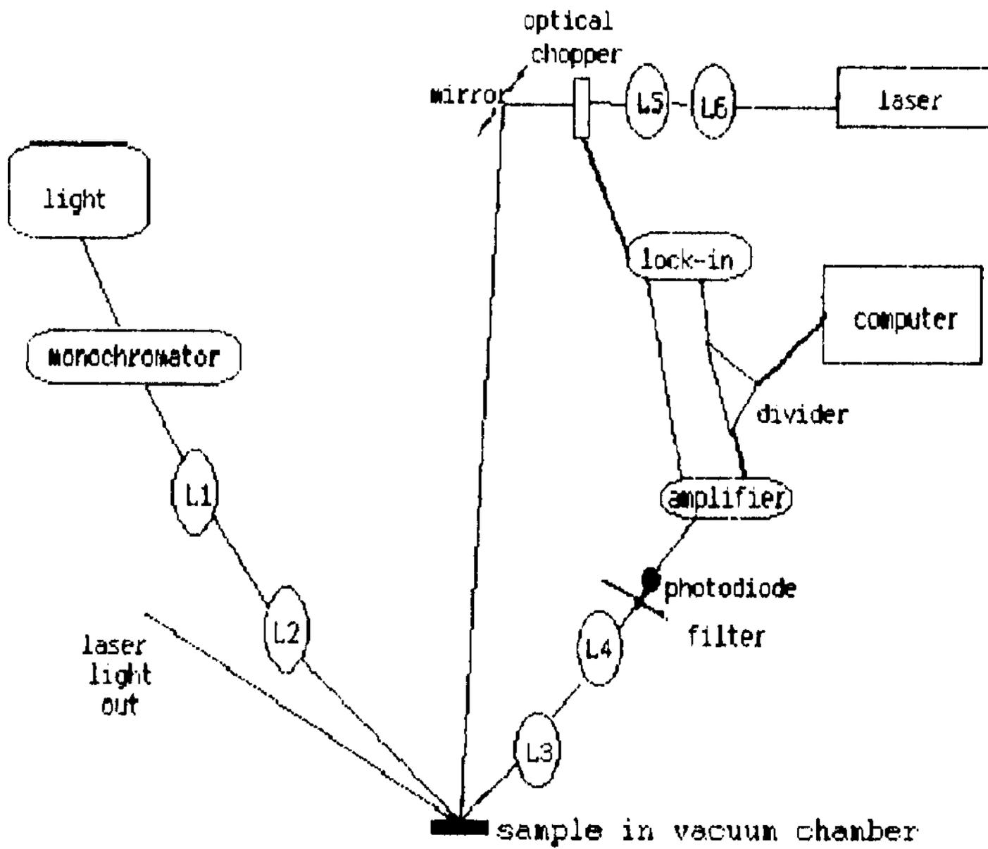
Figure 1 - Photorefectance Apparatus
