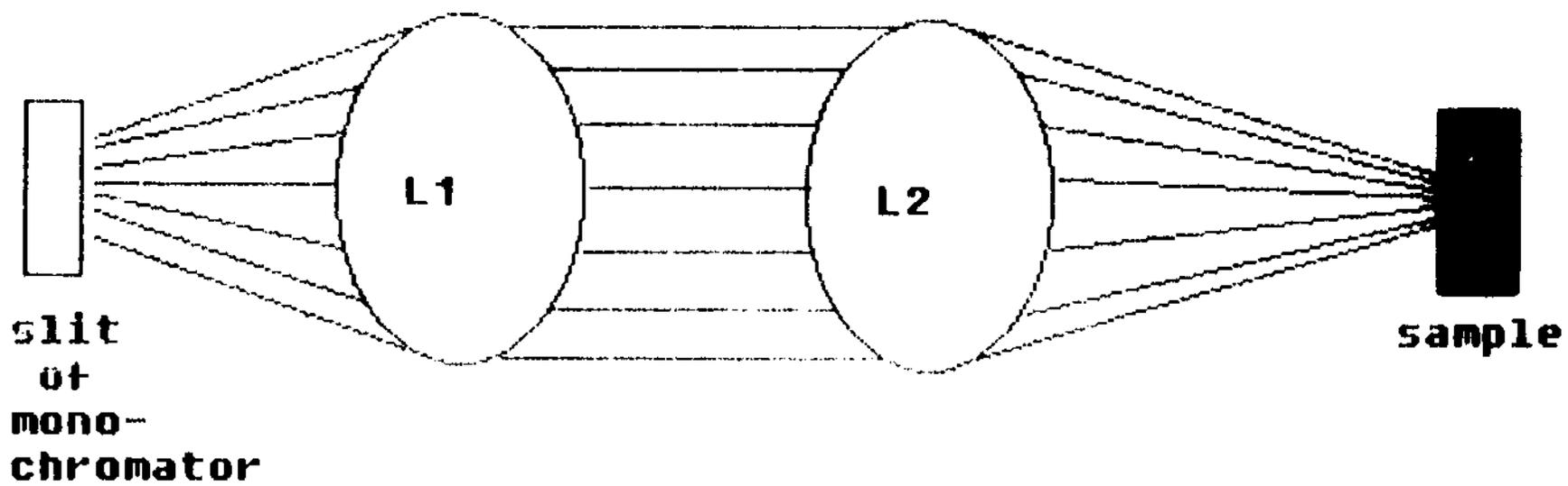
Figure 2 - Lens Arrangement
