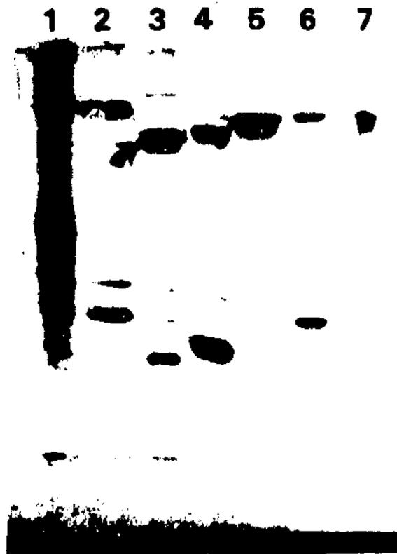
Figure 2. Ten percent native PAGE of methylene- $H_4$ MPT: coenzyme  $F_{420}$  dehydrogenase at six levels of purification. Lane 1, 50 $\mu$ g of CFE protein; lane 2, 30 $\mu$ g of 70% ammonium sulfate; lane 3, 30 $\mu$ g first peak of activity from phenyl-sepharose (with component C +); lane 4, 30 $\mu$ g second peak of activity from phenyl-sepharose (component C separated); lane 5, 20 $\mu$ g methotrexate pool; lane 6, 10 $\mu$ g Mono Q; lane 7, 5 $\mu$ g Superose.
