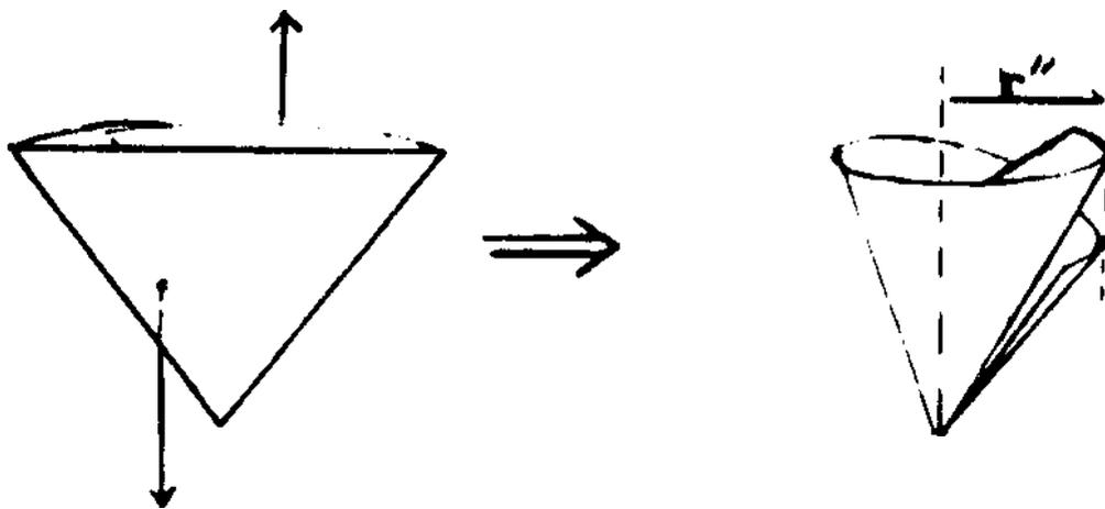
This deformation reduces the radius  $r'$  to  $r''$
