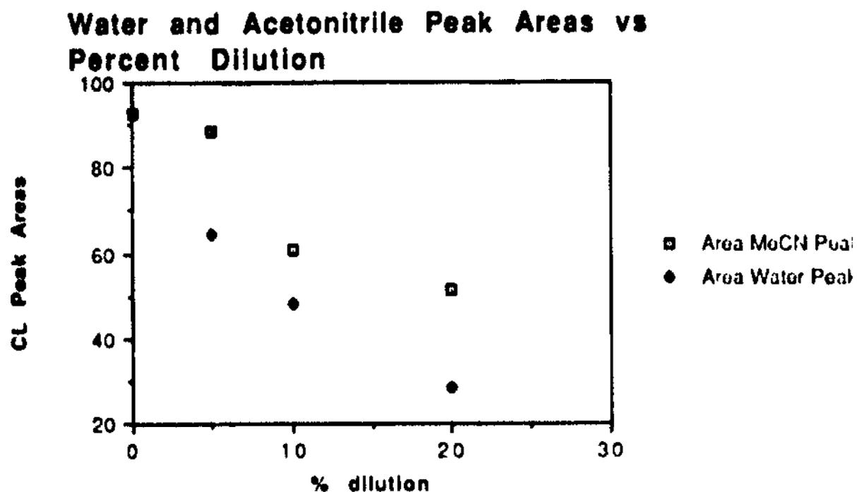
Figure 20 illustrates the acetonitrile and water intensity versus percent dilution data. As mentioned above, the data plotted here was used to produce Figure 10 via the normalization procedure.
