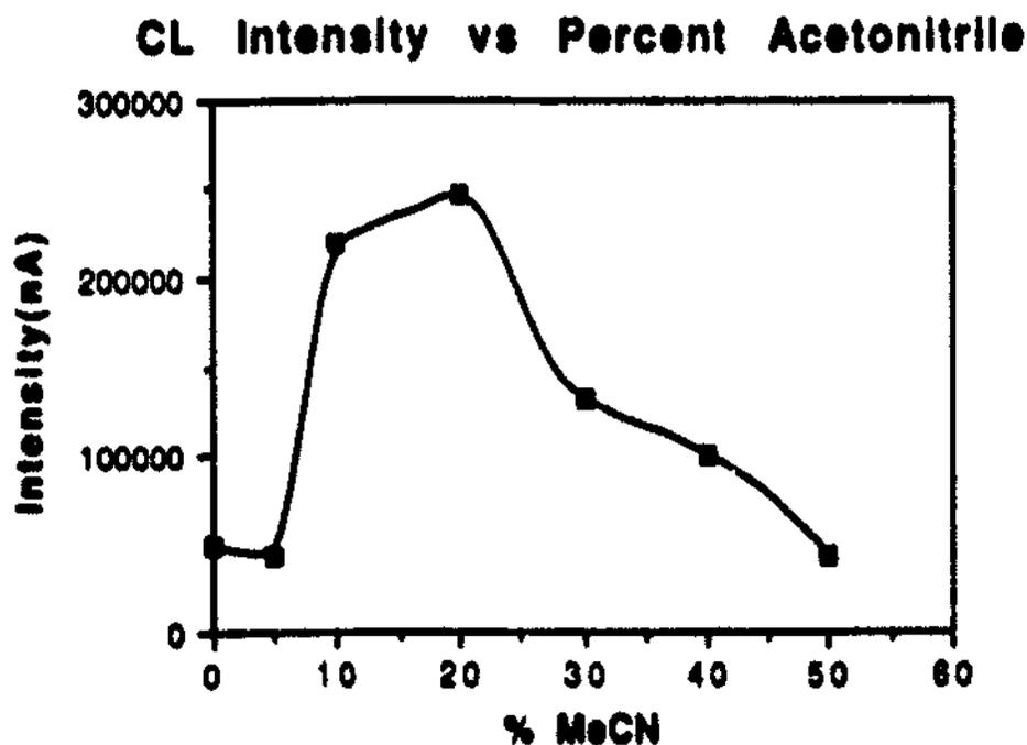
The increase in intensity upon application of 5% acetonitrile is absent in this experiment. In fact there was a slight decrease in emission. However, the general curve shape and magnitudes seen here for 0-20% acetonitrile agree with that seen in Figure 10 over this same solvent composition range. At 20% there is a slight increase, followed by a steady decline in chemiluminescence from 20% to 50%.
