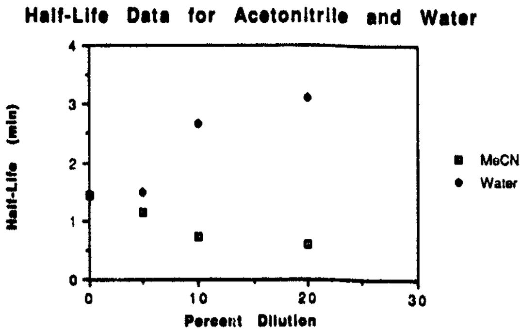
Clearly, with an increase in dilution by water, the half-life of the chemiluminescence was greatly extended. Conversely, a significant decrease in half-life is observed for the acetonitrile system.
