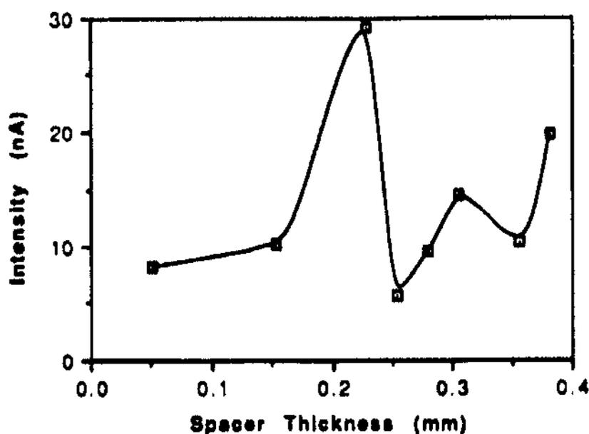
thickness. Increasing spacer thickness has the effect of decreasing the linear flow rate of solution through the cell. This may cause a change in the chemiluminescence due to kinetic factors. Also, the increase in flow
