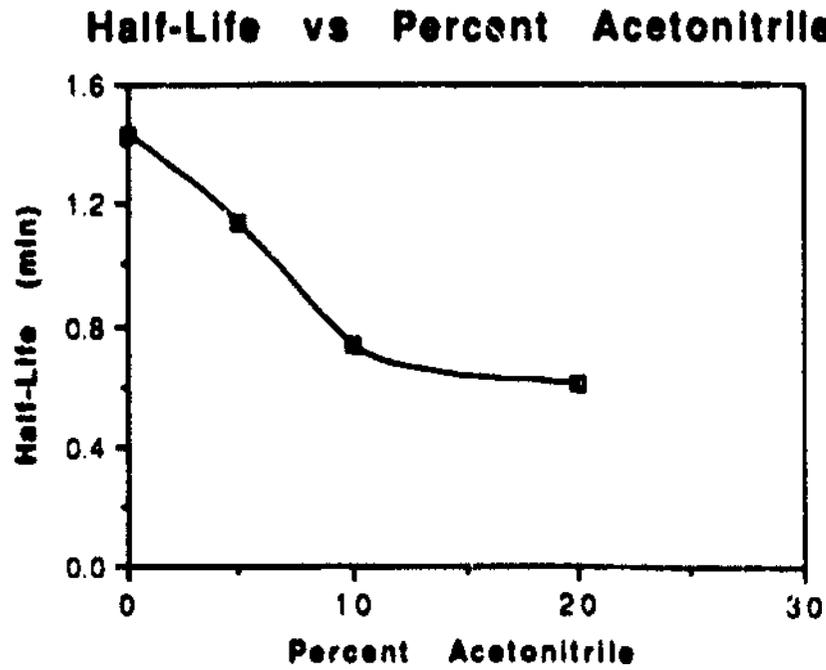
The half-life data decrease sharply from 0% to 10% and then levels off slightly from 10% to 20%. Note that the data indicate half-lives for the acetonitrile system that are significantly shorter than those of the water blanks. A comparison of the raw data is given in Figure 12.
