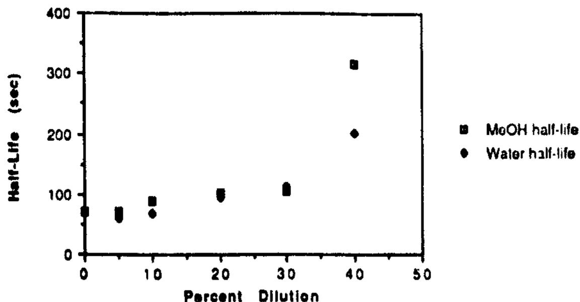
water and methanol dilutions. Note that both are roughly identical with the exception of the 40% data points. The slow increase in half-life seems to be independent of solvent. It is worth noting that from 0% to 30% dilution the half-life increased by 35 seconds (or about 45%), a fact that may have some practical significance in HPLC separations.
