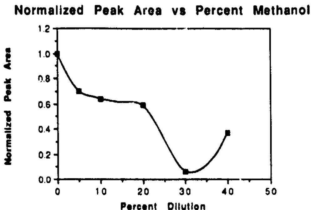
Thus, upon addition of 5% methanol, a 40% decrease in initial intensity and a 40% decrease in the total number of photons emitted is seen. The decrease in peak area may indicate a decrease in the quantum efficiency of the system or a decrease in the rate and/or extent of the CL reaction. In any case, when employing methanol in chemiluminescence-based detection schemes, these factors should be taken into account.
