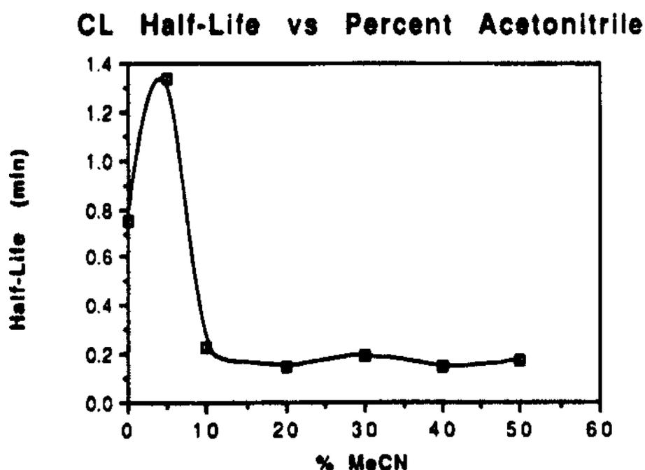
Note the discrepancy for the 0% data points between Figure 17 above and Figures 11 and 12 previously. Although the three data points were taken for a 0% concentration of acetonitrile, the luminol, hemin, and peroxide concentrations differed between Figure 17 and Figures 11 and 12. In order to eliminate the need for normalization of the data, the concentration of luminol in the 0-50% experiment was constant at 50  $\mu$ M in all solutions,
