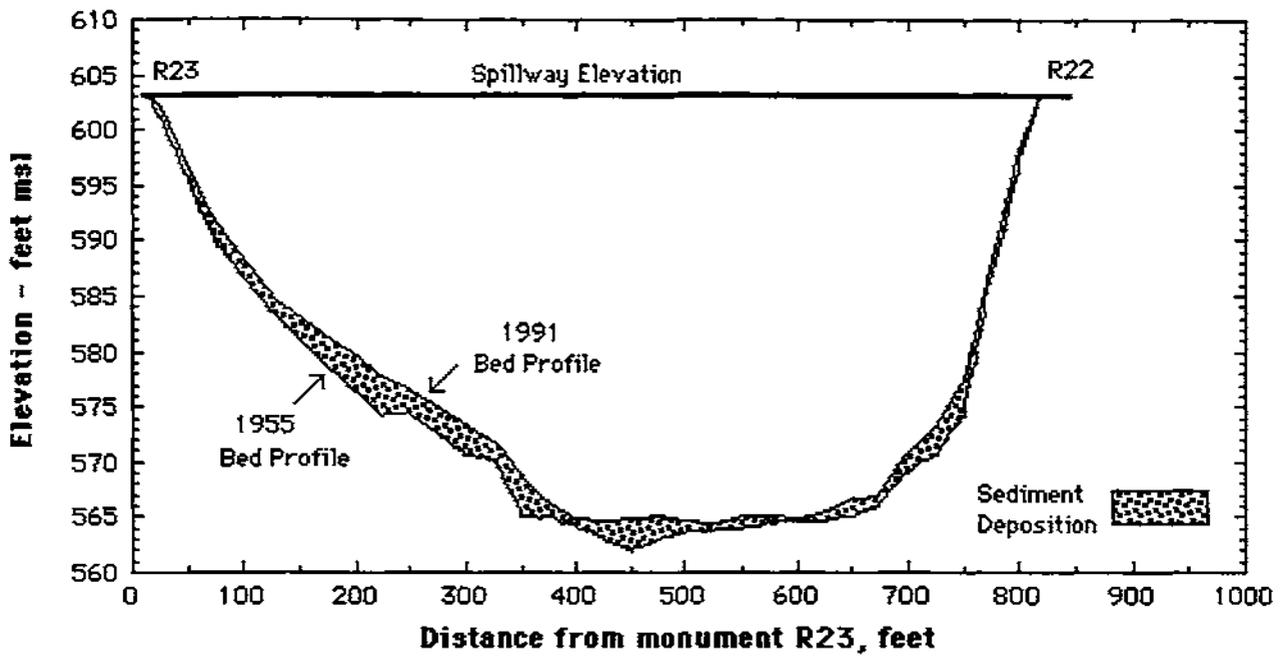
Figure 3. Typical cross section of Siloam Springs Lake near the dam
