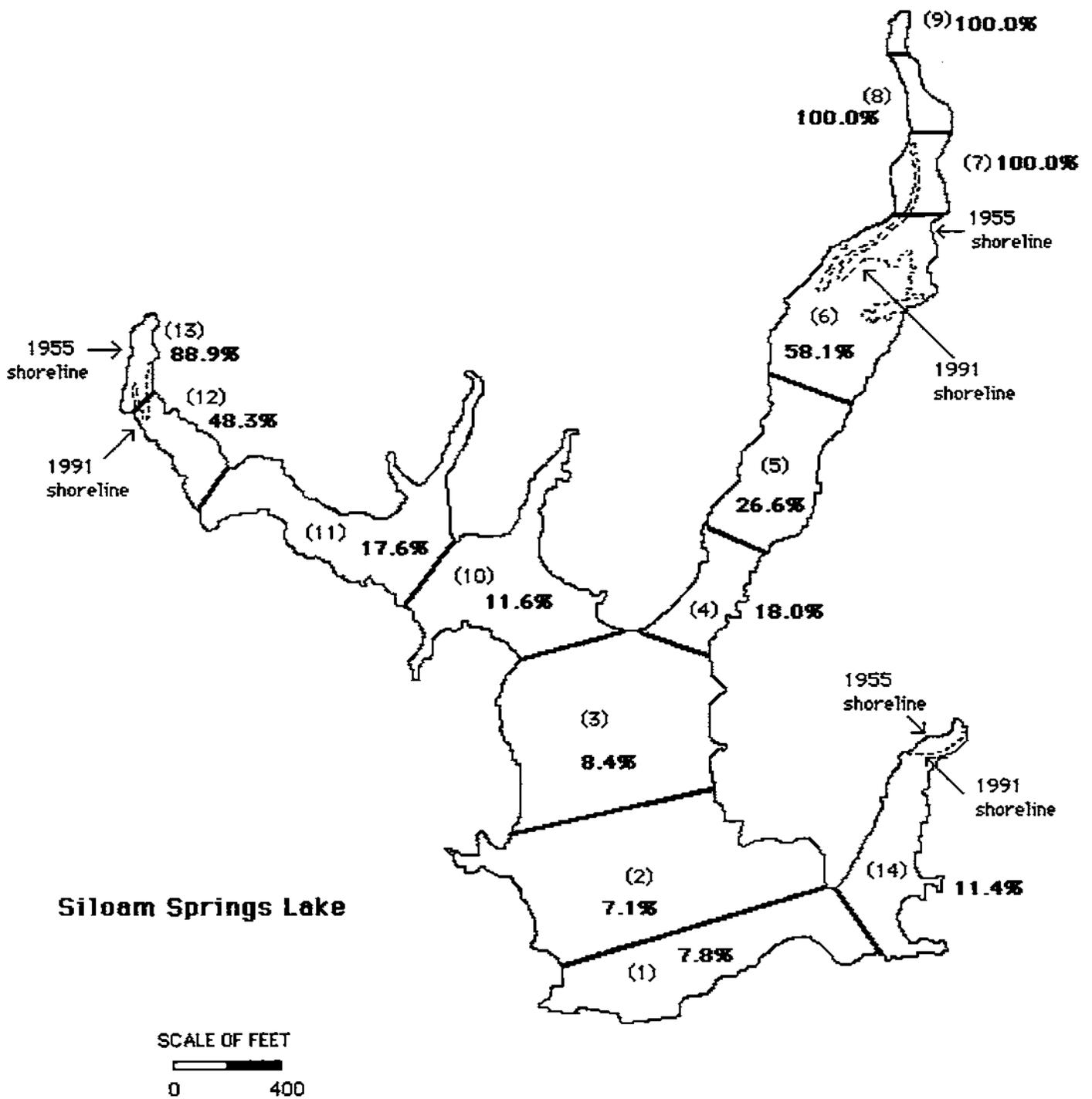
Figure 5. Percent loss of original lake volume by lake segment and changes in shoreline for Siloam Springs Lake
