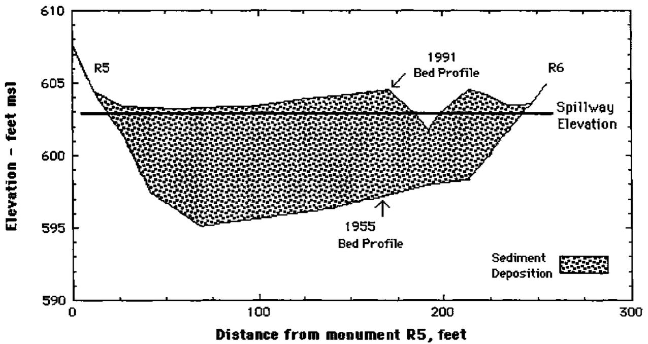
Figure 4. Typical cross section of Siloam Springs Lake illustrating sediment deposition above the spillway elevation
