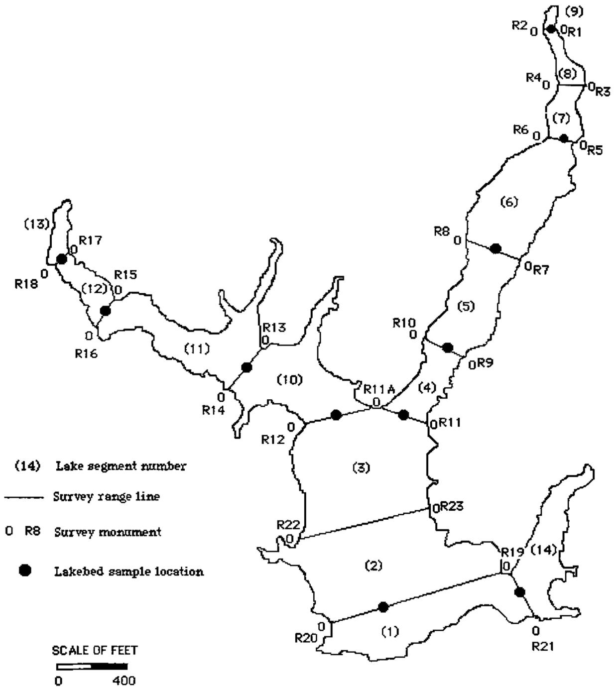
Figure 2. Siloam Springs State Park lake survey range lines, survey monuments, lake segments, and lakebed sample locations
