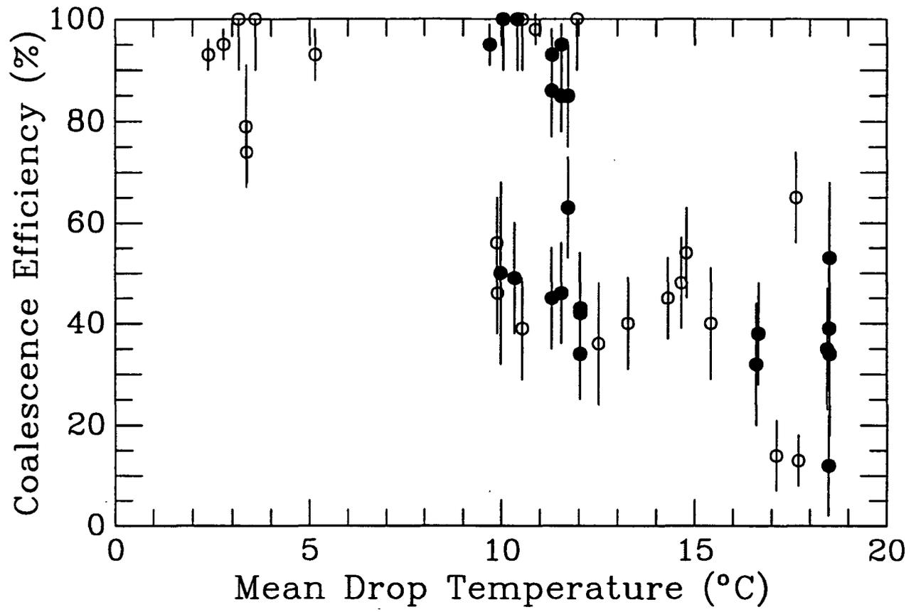
Figure 2. Experimentally determined coalescence efficiency versus mean drop temperature.
