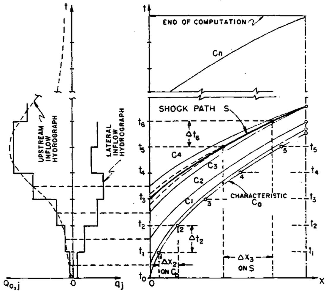
Figure 3. Tracing characteristics and shock paths in kinematic wave routing (after Borah et al., 1980)
