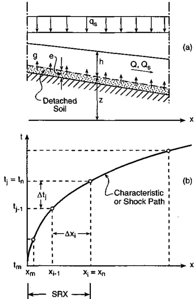
Figure 4. Sediment routing in a flow element: (a) schematic flow element: (b) tracing characteristic or shock path (after Borah, 1989b)
