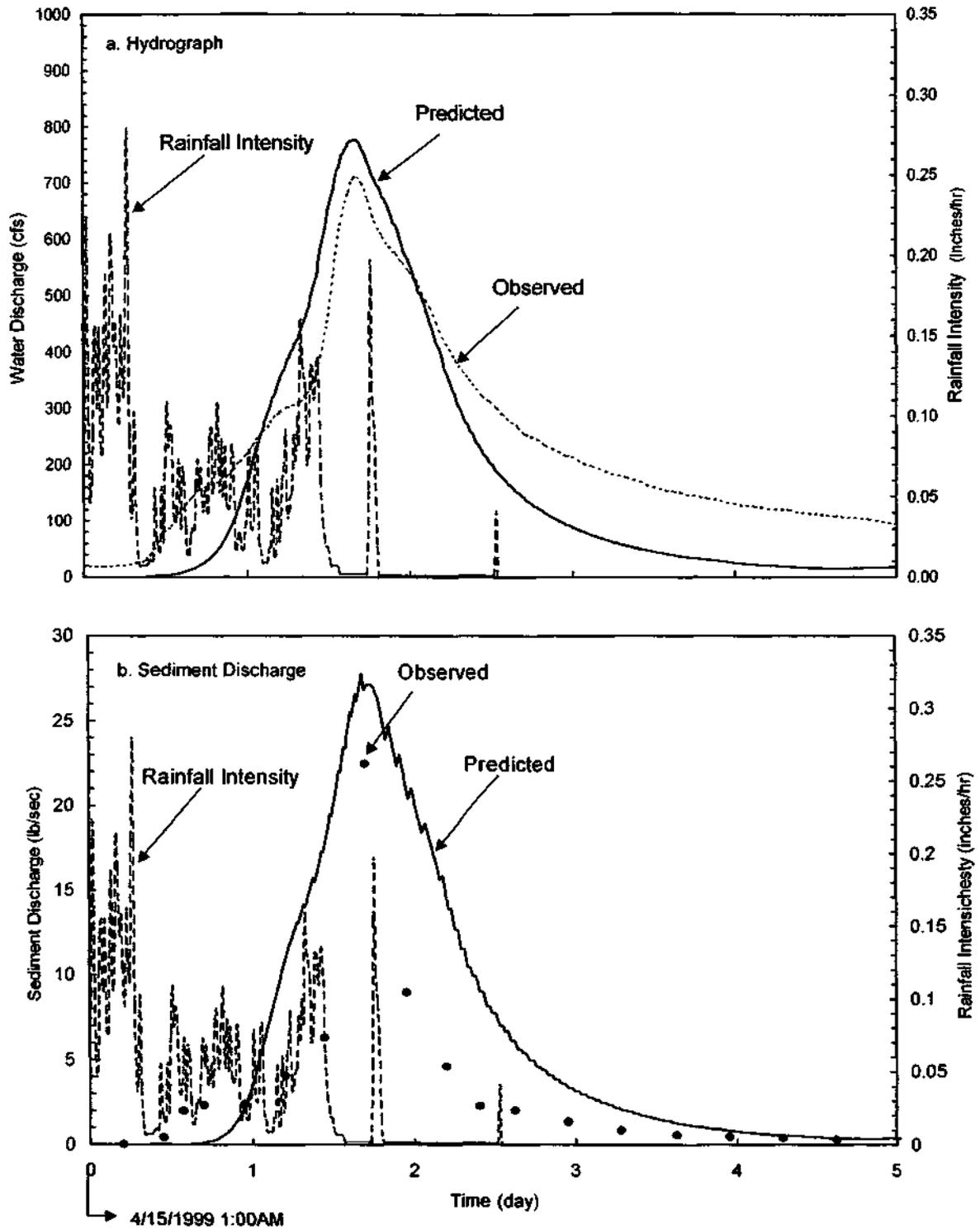
Figure 32. Comparison of observed and predicted (a) hydrograph and (b) sediment discharge at Big Ditch station for storm on April 15-16, 1999
