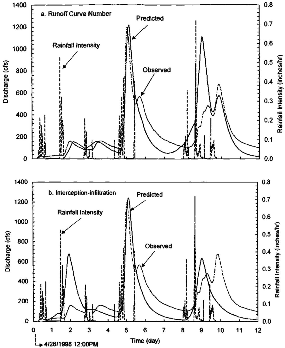
Figure 29. Comparison of observed and predicted hydrographs (using rainfall excess procedure) at Big Ditch station for storms in April-May 1998:
