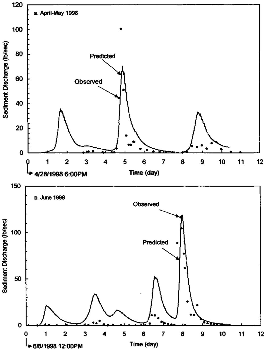
Figure 31. Comparison of observed and predicted sediment discharges at Big Ditch station for storms during (a) April-May 1998 and (b) June 1998
