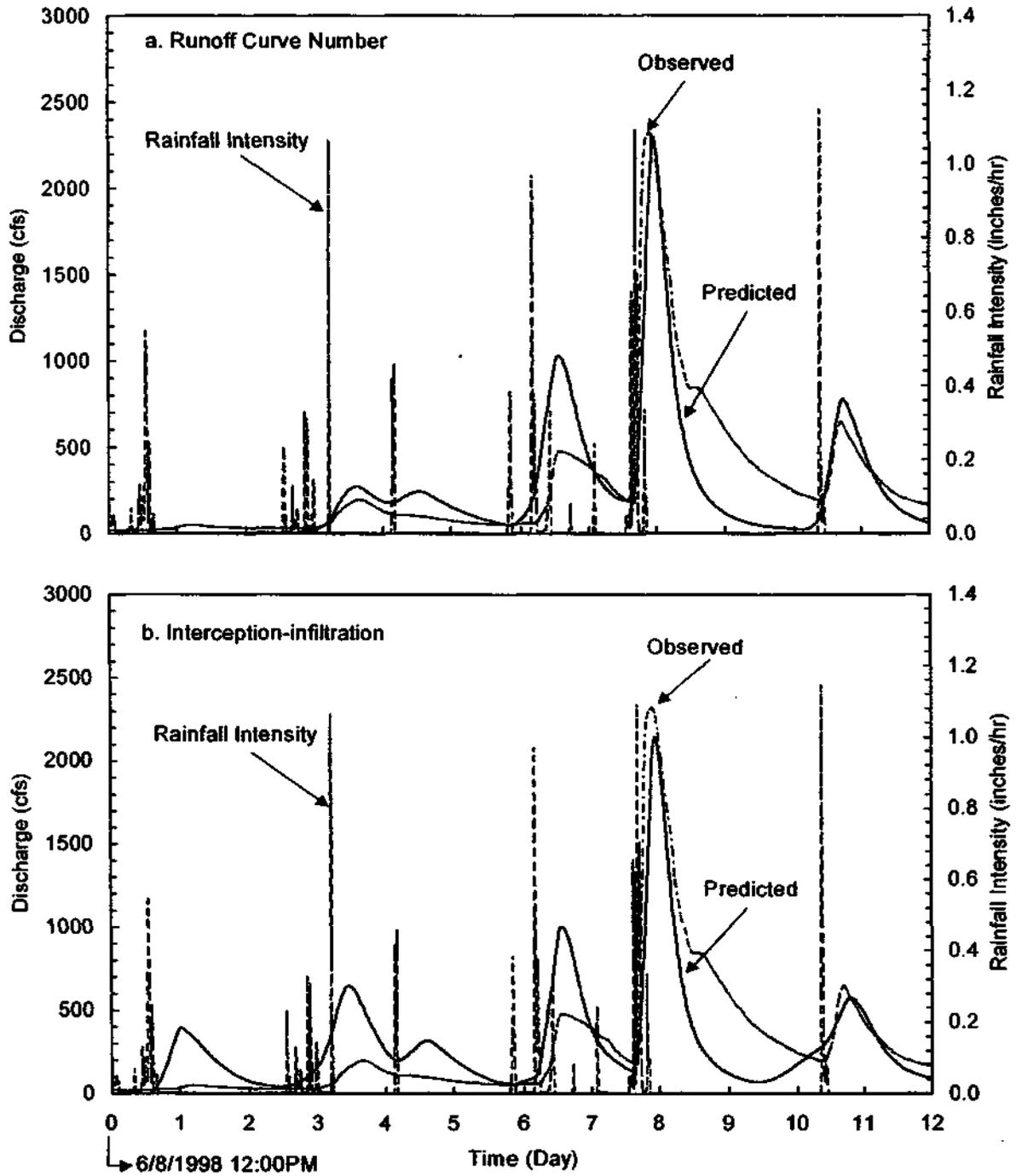
Figure 30. Comparison of observed and predicted hydrographs (using rainfall excess procedure) at Big Ditch station for storms in June 1998:
