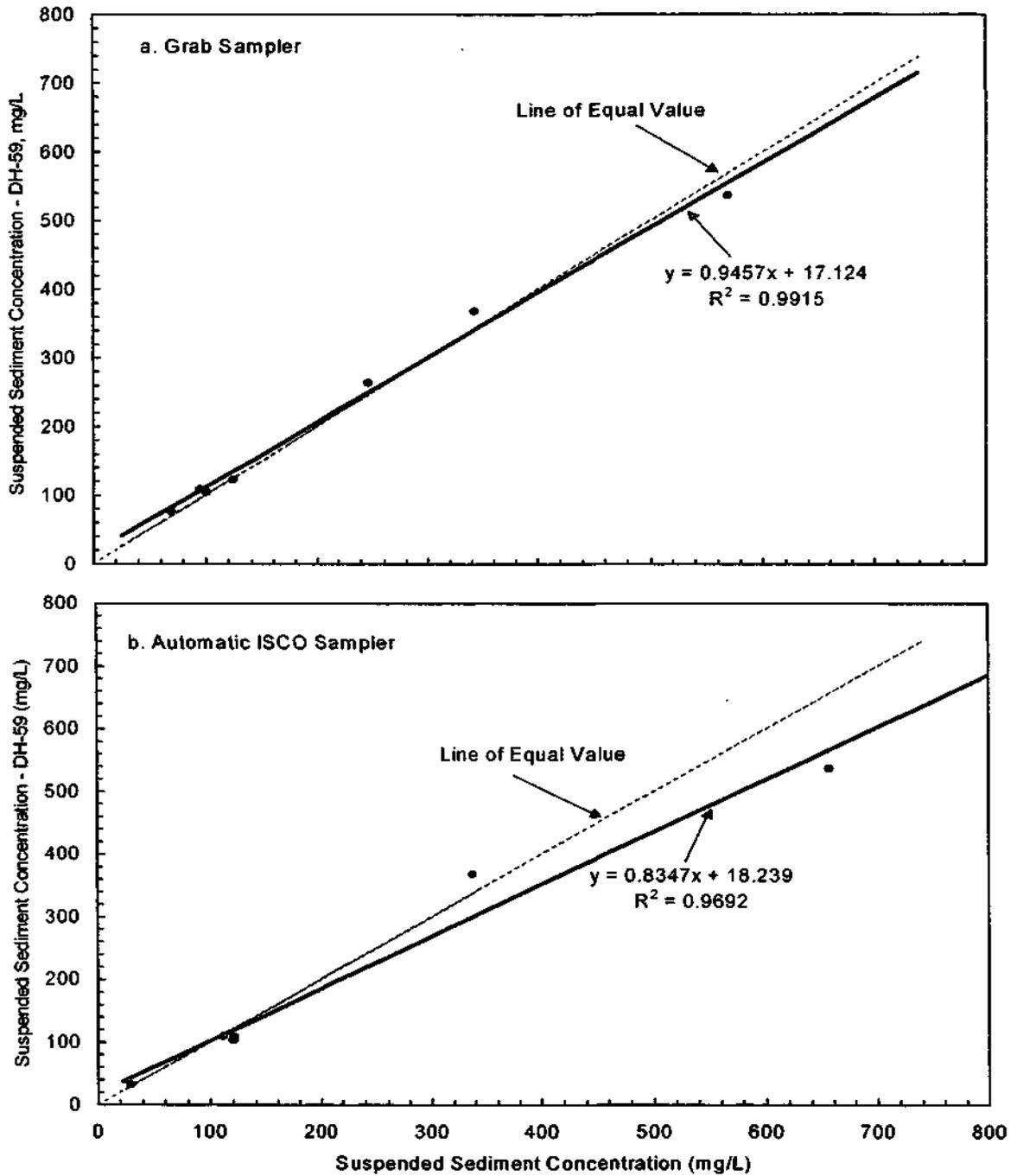
Figure 19. Comparison of suspended sediment concentration measured by depth integrated DH-59 sampler and by (a) grab sampler and (b) automatic ISCO sampler
