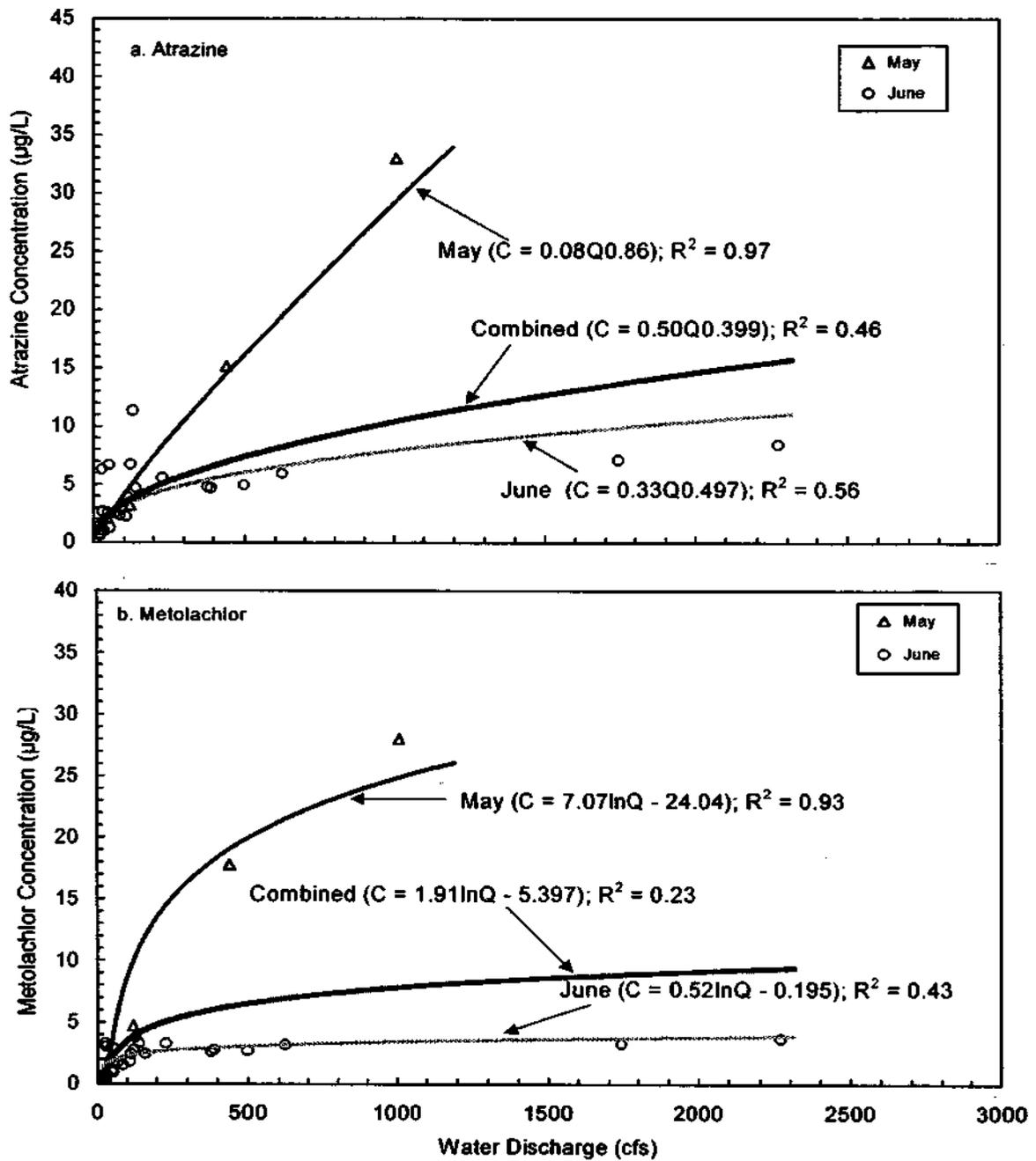
Figure 23. Correlation of herbicide concentrations with water discharge at the Big Ditch station based on observations made during Spring 1998 storms:
