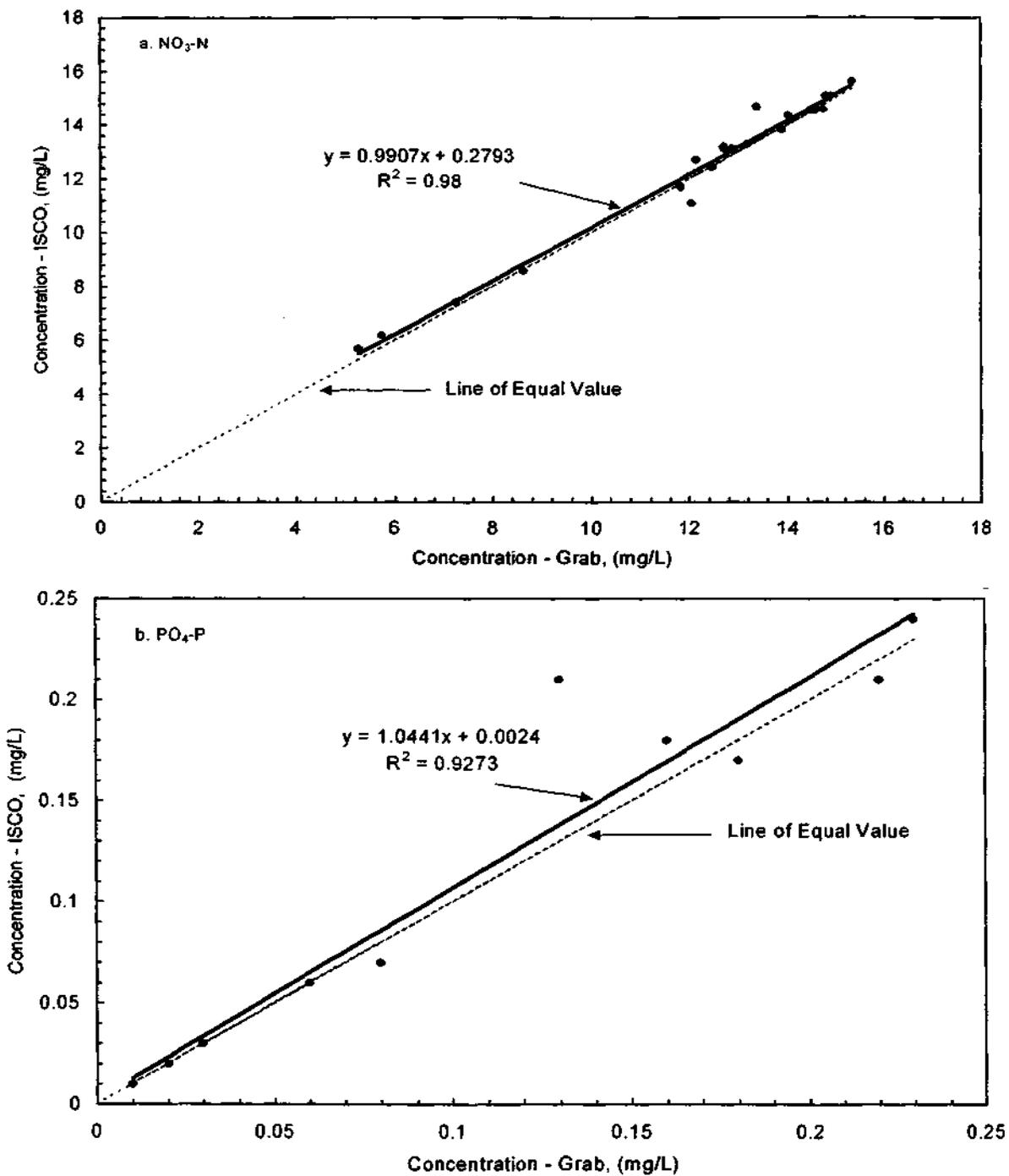
Figure 18. Comparison of concentration measurements by automatic ISCO and grab samplers for (a) nitrate-nitrogen and (b) phosphate-phosphorous
