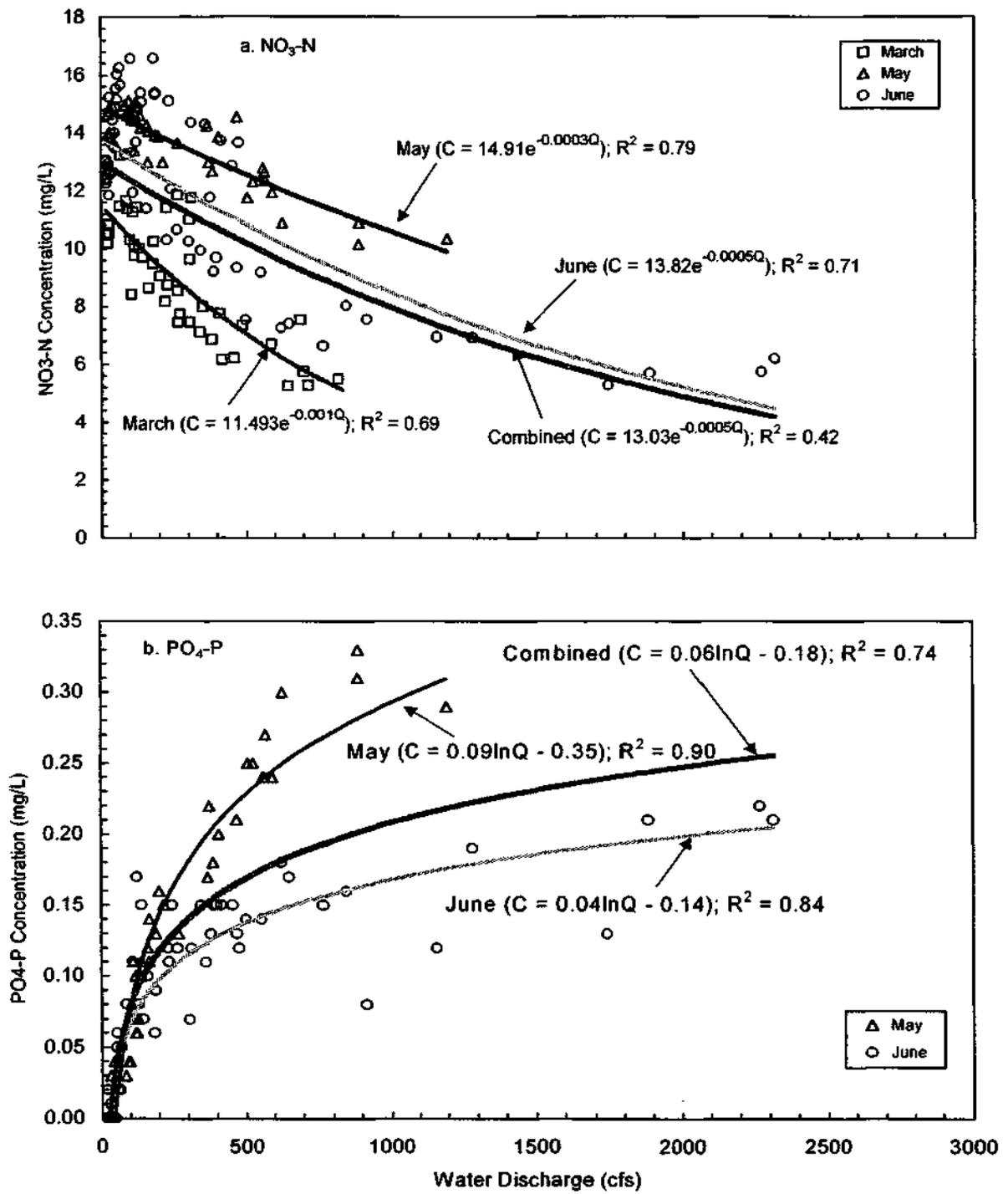
Figure 22. Correlation of nutrient concentrations with water discharge at the Big Ditch station based on observations made during Spring 1998 storms:
