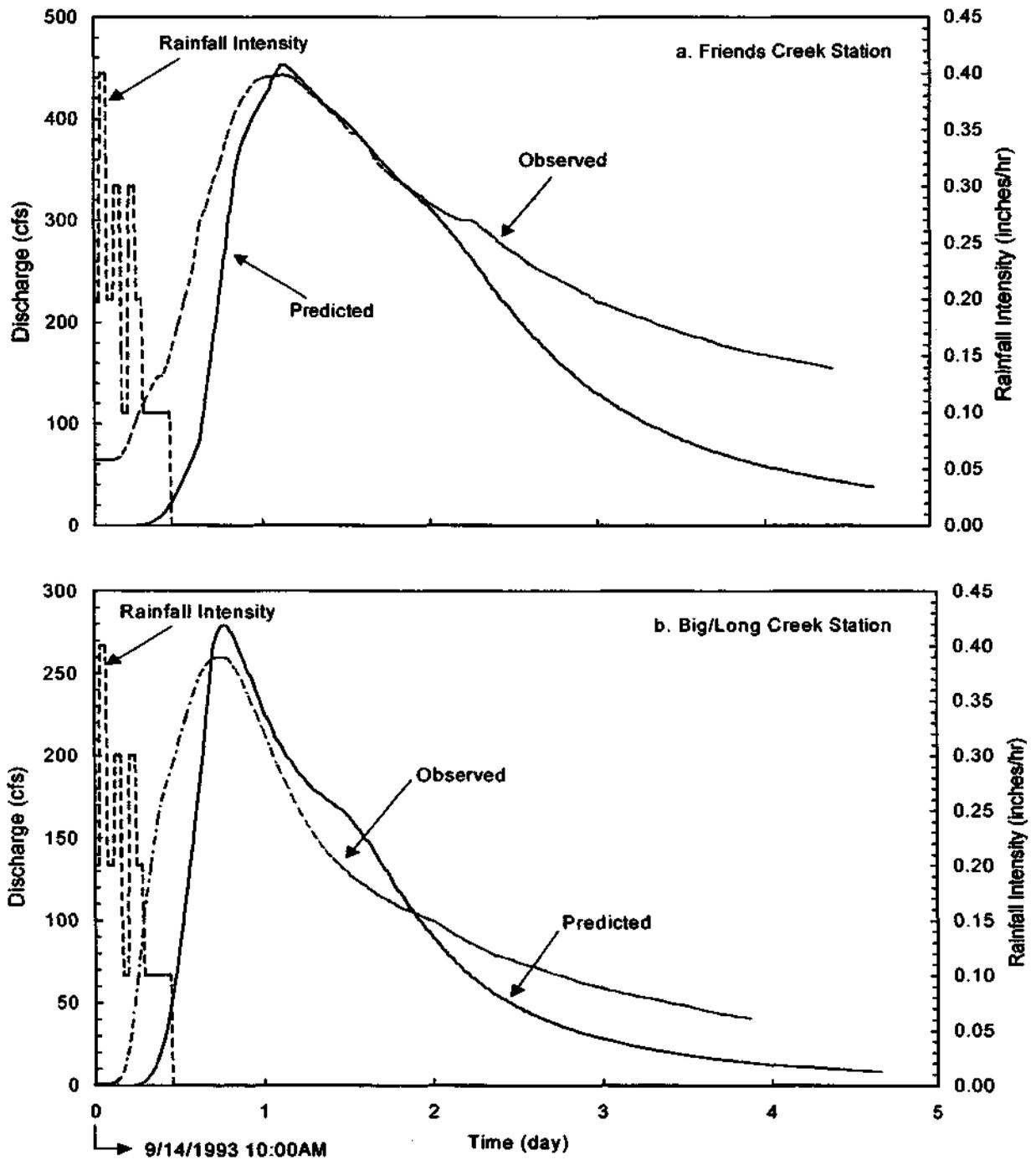
Figure 26. Comparison of hydrographs for September 14, 1993 storm at (a) Friends Creek station and (b) Big/Long Creek station
