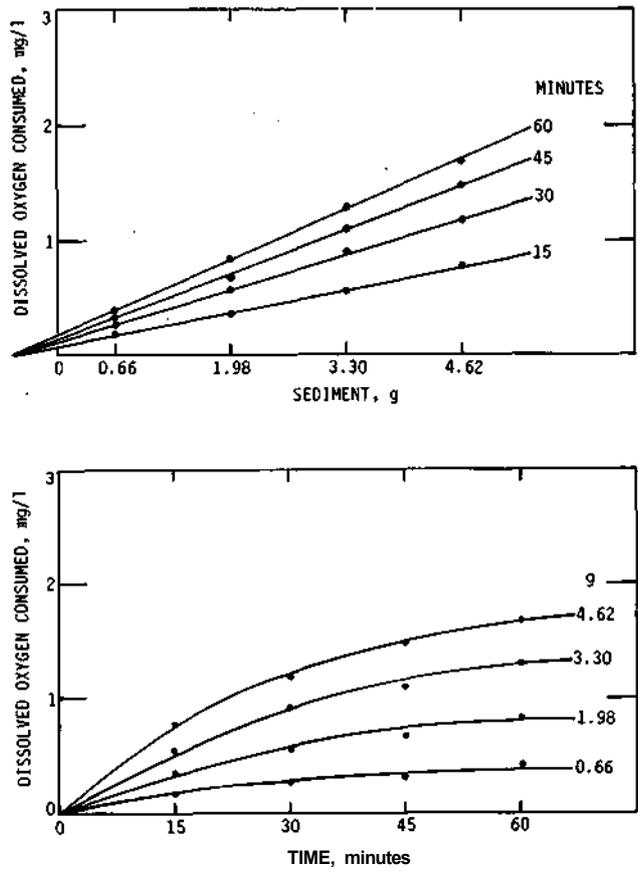
Figure 33. Relationship of oxygen consumed and amount of sediment dosage introduced
