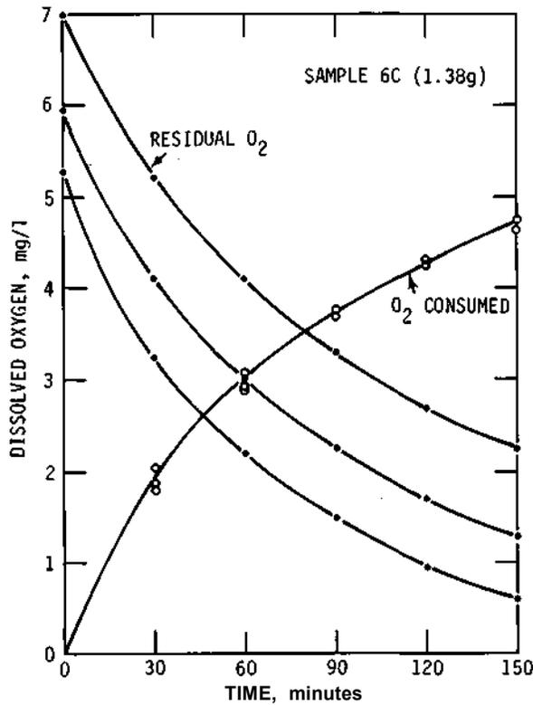
Figure 31. The effects of initial dissolved oxygen levels on oxygen consumed by sediments
