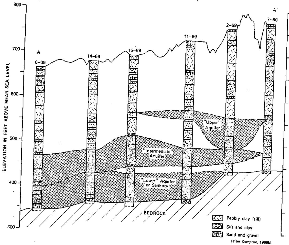
Figure 2. Geologic cross section of the valley fill (after Kempton, 1969b)
