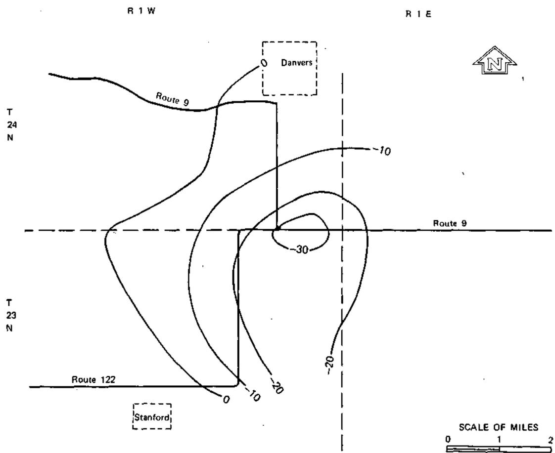
Figure 8. Changes in water levels by April 1981 in wells tapping the lower and intermediate aquifers
