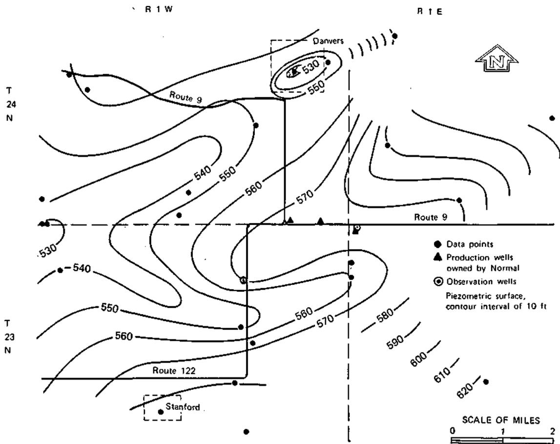
Figure 6. Approximate piezometric surface of the lower and intermediate aquifers immediately before development
