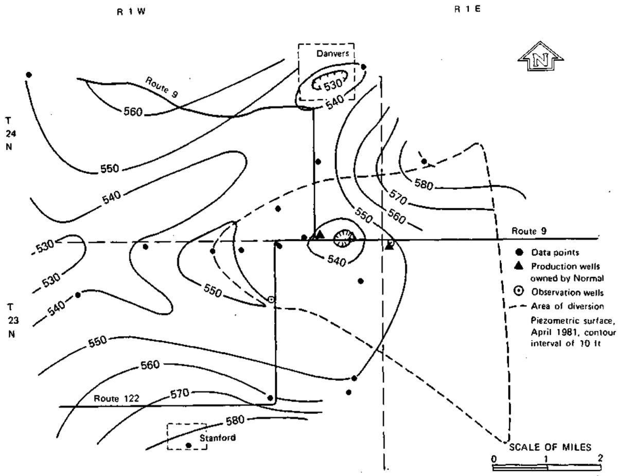
Figure 7. Approximate piezometric surface of the lower and intermediate aquifers, April 1981, and area of diversion
