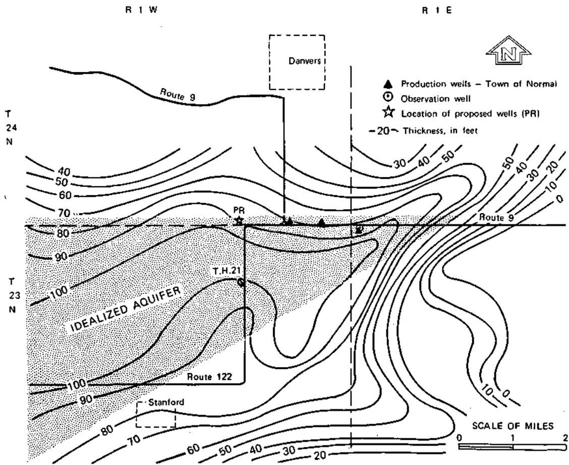
Figure 9. Combined thickness of the lower and intermediate aquifers
