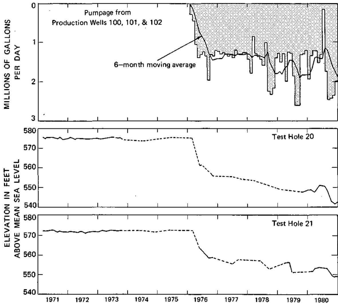
Figure 5. Pumpage and water levels in the Normal west well field
