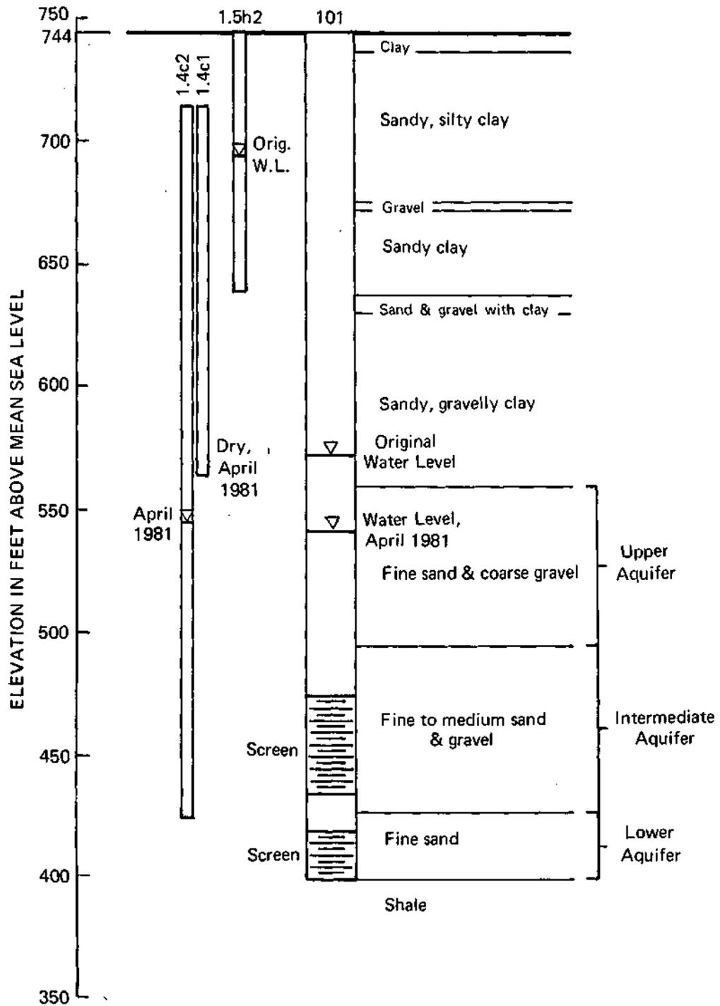
Figure 4. Simplified log of Production Well 101 and examples of domestic wells in surficial (1.5h2), upper (1.461), and intermediate (1.4c2) aquifers
