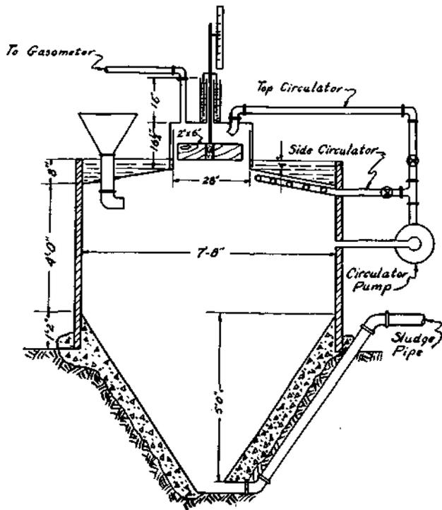
Digester Equipped for Scum Wetting to Equalise Alkalinity and Speed Digestion
