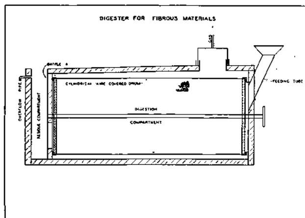
The Drum-Screen Digester for Fibrous and Scum Forming Materials
