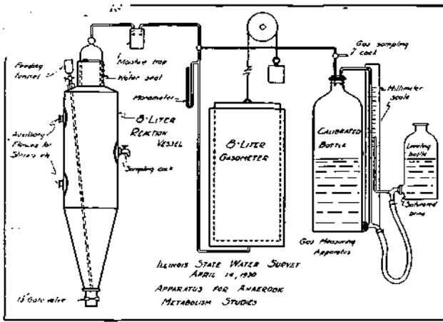
Laboratory Equipment Used in Anaerobic Digestion and Stabilisation Studies
