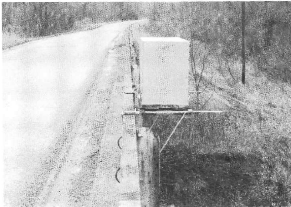
Figure 9. USGS California-type sediment sampling box
