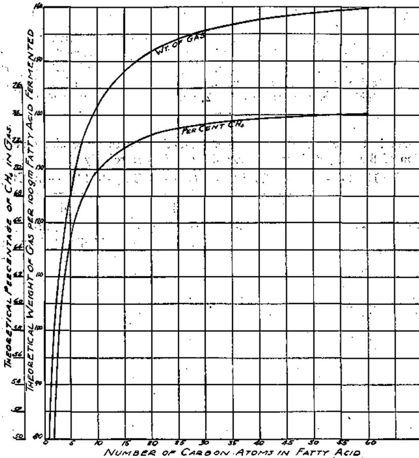
Fig. 4—Theoretical weight and methane content of fermentation gases.
