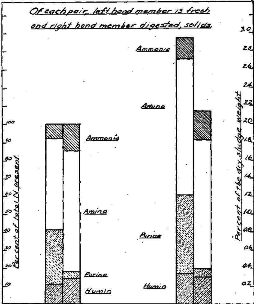
Fig. 1—Ammonia, amino, purine, and humin nitrogen in hydrolyzed sewage protein. Plotted as per cent of total nitrogen present (left) and as per cent of dry sludge weight (right).
