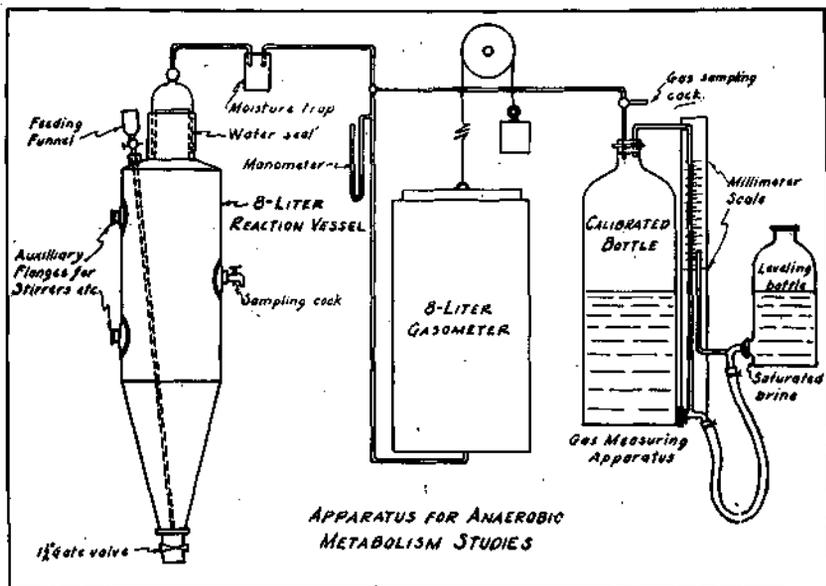
Figure 3.—Apparatus for Anaerobic Digestions.
