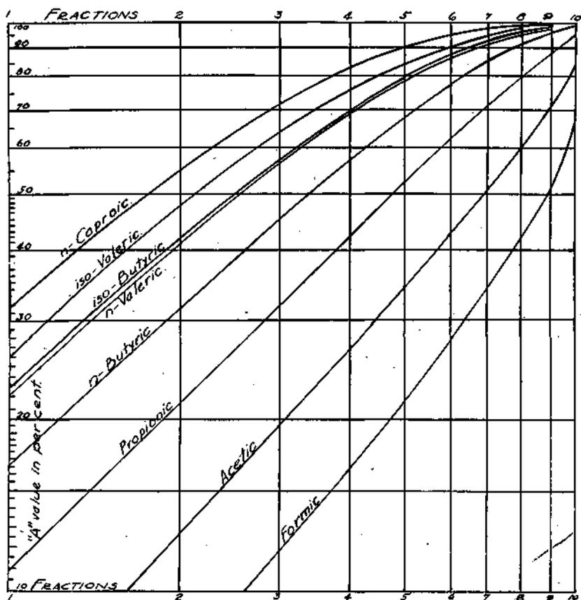
Fig. 5--Duclaux distillation curves.
