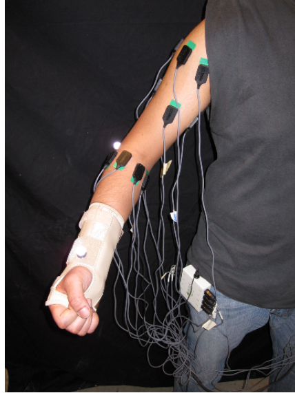
Figure 2.1: Placement of EMG electrodes on subject.
