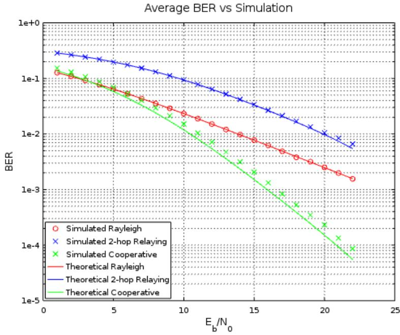
Figure 2.2:  $\bar{P}_\epsilon$  in Cooperative Communication ( $\sigma_{SR}^2 = \sigma_{SD}^2 = \sigma_{RD}^2 = 1$ )
