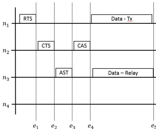
Figure 3.5: Handshaking Between Nodes with Cooperation in  $\mathbf{G}_1$
