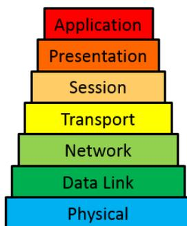
Figure 1.2: OSI 7 Layer Protocol Stack
