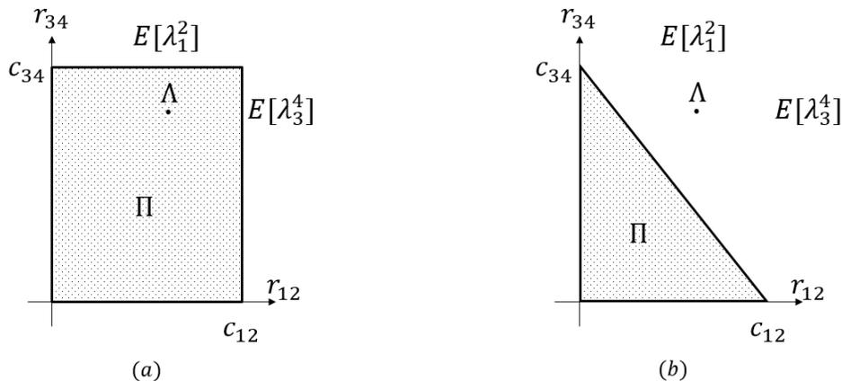
Figure 3.3: Capacity Regions of  $\mathbf{G}_1$  with Scheduling Constraints
