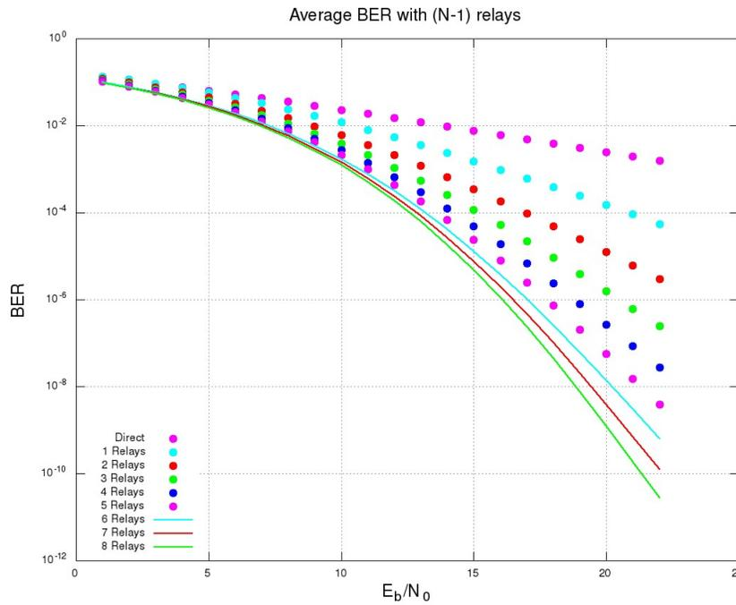
Figure 2.3:  $\bar{P}_\epsilon$  in Cooperative Communication with Multiple Relays
