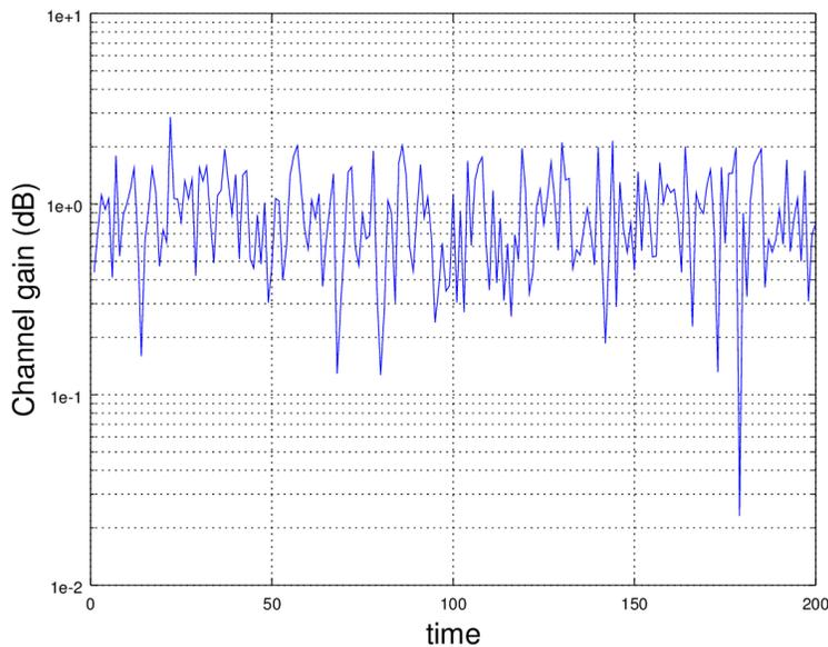
Figure 1.1: Instantaneous Channel Gain Under Rayleigh Fading Conditions
