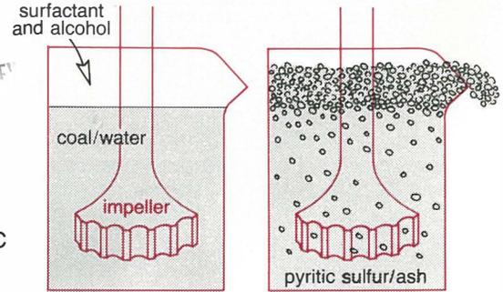
*"We mix finely ground coal with water, then add the surfactants and alcohol. Coal particles are basically floated by bubbles, forming a black froth that we skim off."*
