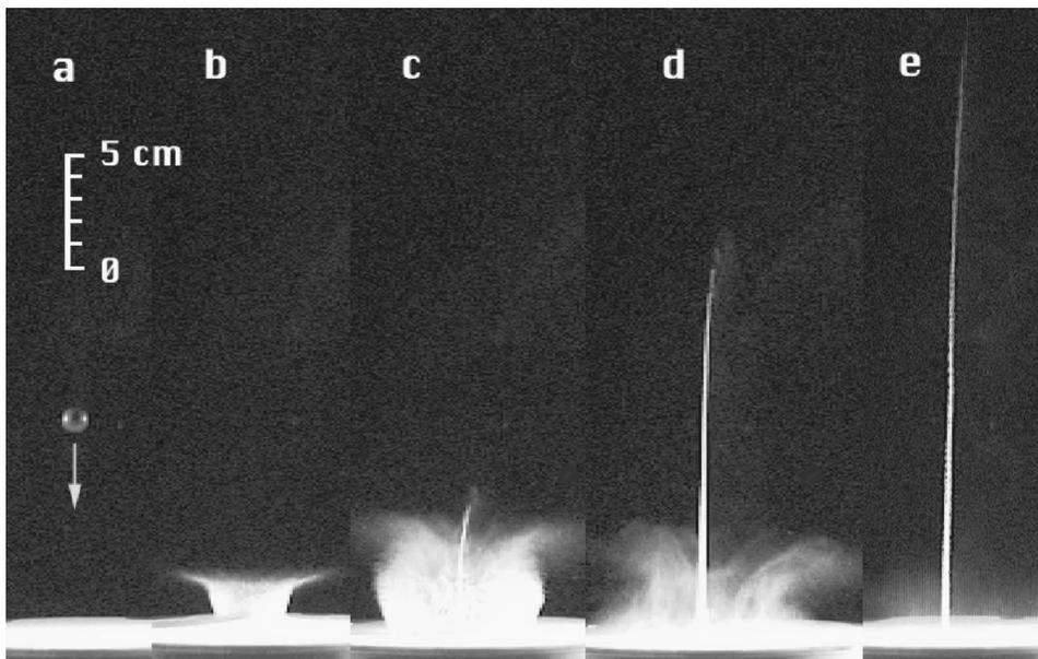
FIG. 1. Granular jet generated by the impact of a lead sphere ( $U=5.5$  m/s,  $D_b=1.34$  cm,  $\rho_b=11.5$  g/cm<sup>3</sup>) onto a deep layer of granular medium, consisting of spherical glass beads 0.080 mm in diameter. The medium sits in a circular glass container 12.2 cm deep and 18.8 cm in diameter. (a)  $t=-18$  ms; (b)  $t=25$  ms; (c)  $t=92$  ms; (d)  $t=160$  ms; (e)  $t=260$  ms. The upward speed of the granular jet is about one-third of the sphere impact velocity.
