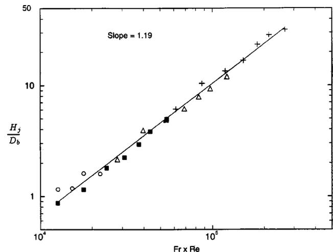
FIG. 3. The dimensionless plot of the maximum height attained by the granular jet, versus the jetting parameter  $Fr \times Re$ . Granular media consist of spherical glass beads with four different mean diameters:  $d_s=0.080$  mm (+), 0.118 mm ( $\Delta$ ), 0.176 mm ( $\blacksquare$ ), and 0.275 mm ( $\circ$ ).
