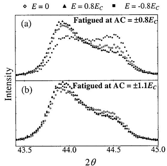
FIG. 3. The pseudocubic (200) profiles at different static electric fields for specimens after cyclic electric fields (AC, 50 Hz,  $10^5$  cycles): (a) at AC  $\pm 0.8 E_C$ , (b) at AC  $\pm 1.1 E_C$ .
