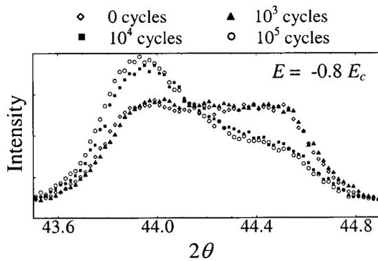
FIG. 4. Effect of the number of cycles of electric fields (AC, 50 Hz,  $\pm 1.1E_C$ ) on the pseudocubic (200) profiles at a static electric field  $E = -0.8E_C$ .
