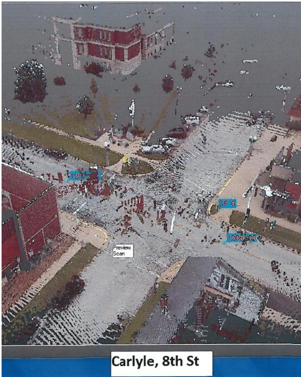
Figure 2: Contract No. 76H11, ADA ramps on US 50, 8th Street intersection generated from laser scanner point cloud with image superimposed.
