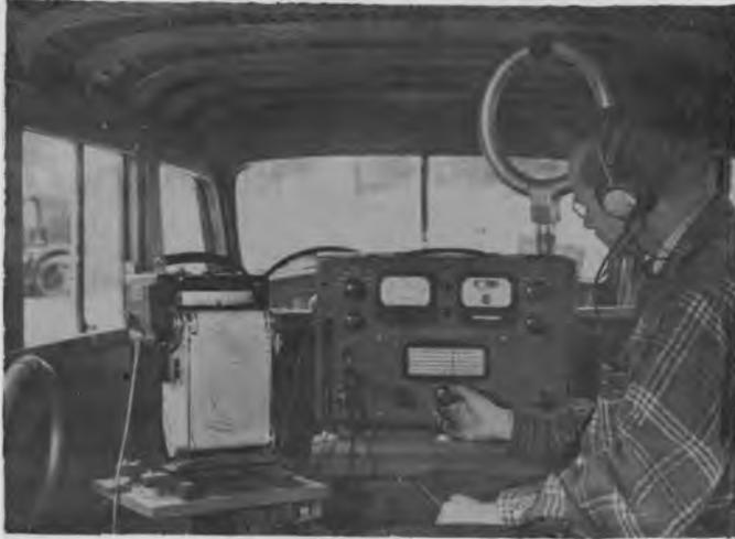
Fig. 1 (left): Illinois Geological Survey mobile field intensity equipment used for measuring radio wave signal strength.
