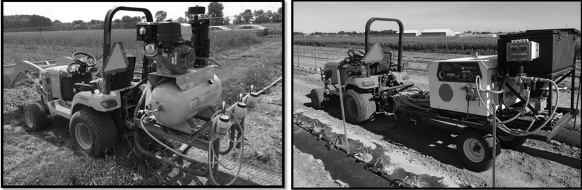
Figure 1.1: Experimental abrasive grit applicators used in 2015 (left) and 2016 (right).
