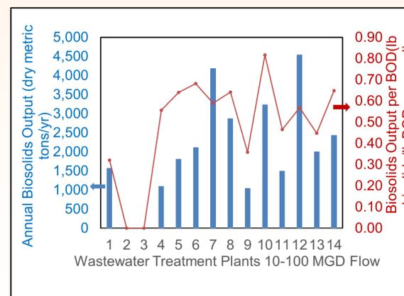
Fig. 3: Annual biosolids output and biosolids output per unit of BOD removed from influent water. Biosolids include both waste activated sludge and digested solids. Lower output biosolids to removed BOD is better
