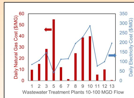
Fig. 2: Daily electricity and natural gas cost per MG treated. Electricity costs dominate treatment costs.
