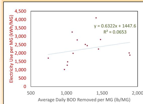
Fig. 1: Poor correlation between electricity use and BOD removal per MG treated indicates wide variation in energy efficiency.
