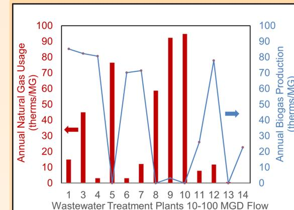
Fig. 4: Annual natural gas usage and biogas production. Lack of biogas recovery and usage increase natural gas use.
