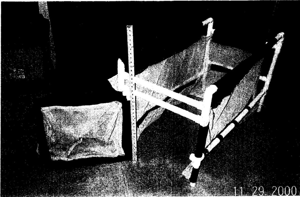
Figure 1: Benthic sampler used to estimate population size of mottled sculpin (*Cottus bairdi*) in Black Partridge Creek. The sampler is  $5.38\text{in}^2$  ( $1/2\text{m}^2$ ) in area.
