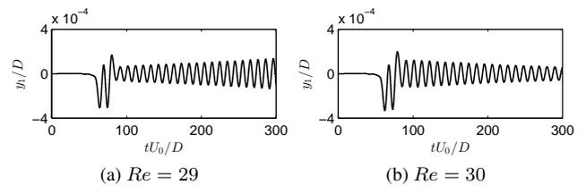
Figure 2: Time series with decaying and growing solutions at the beginning of the synchronization  $Re_c$  for  $1/F_n^* = 0.35$  of the cylinder without NES.
