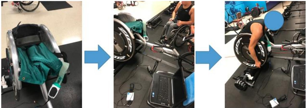
**Figure 1. Pressure mat system measuring pressure skin pressure on the kneeling tray**
