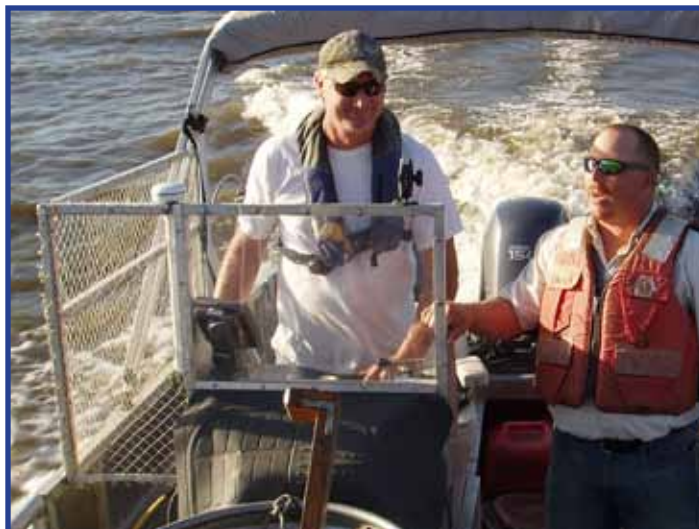
A boat rigged with a protective net and Plexiglas™ shield to protect the operator.
