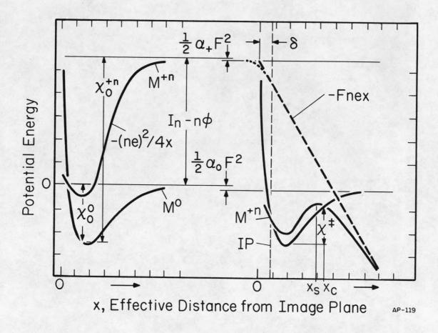
Fig. 2 Potential curves for charge exchange model of field evaporation.  $x_c$  = point of intersection for atomic and ionic curves. The half-width  $\Gamma$  due to interaction between the curves is not indicated.
