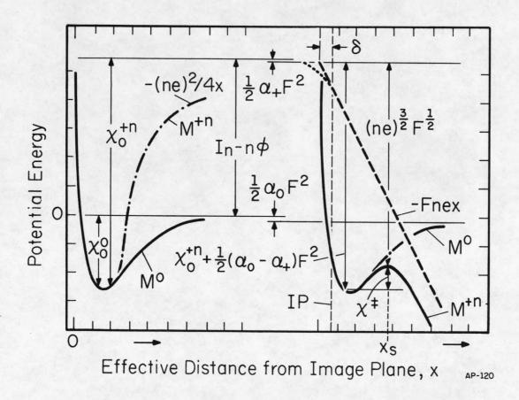
Fig. 1 Schematic potential diagram for the field evaporation of a metal according to the image potential model.  $M^{\circ}$  = neutral metal atom;  $M^{\dagger n}$  = metal ion with charge +n.  $\chi^{\ddagger}$  = activation energy for field evaporation; IP = image plane;  $\delta$  = screening length;  $\kappa$  = location of Schottky hump.
