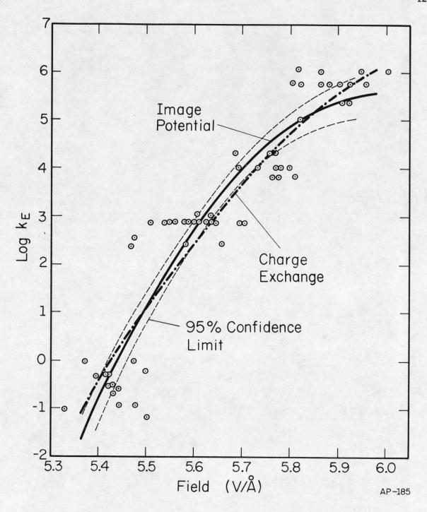
Fig. 3 Rate of field evaporation for W adatoms from W(110). Charge exchange curve - data fitted by Eq.(8); Image potential - data fitted by Eq.(7), with n = +2. Experimental data-set TT10, Reference 11.
