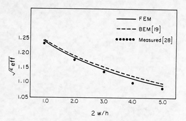
Figure 11.  $\sqrt{\varepsilon_{\it{eff}}}$  of shielded inverted microstrip line versus shape ratio 2w/h.
