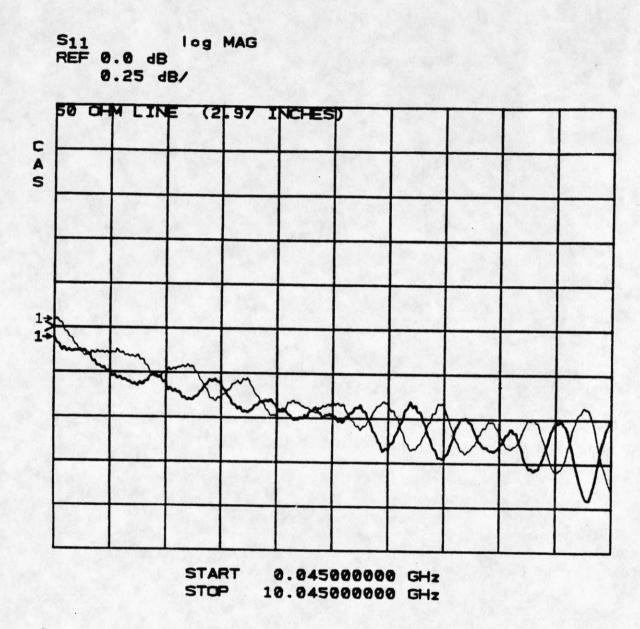
Figure 15. Frequency-domain measured results of  $S_{11}$  parameter.
