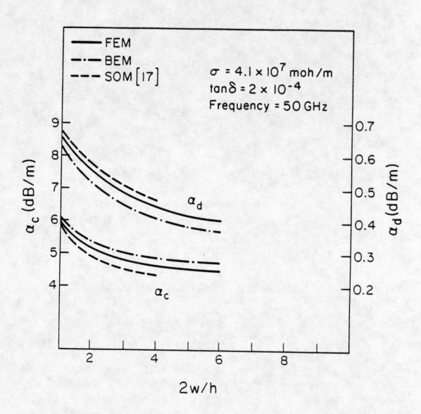
Figure 12. Dielectric and conductor losses of shielded inverted microstrip line versus shape ratio 2w/h.
