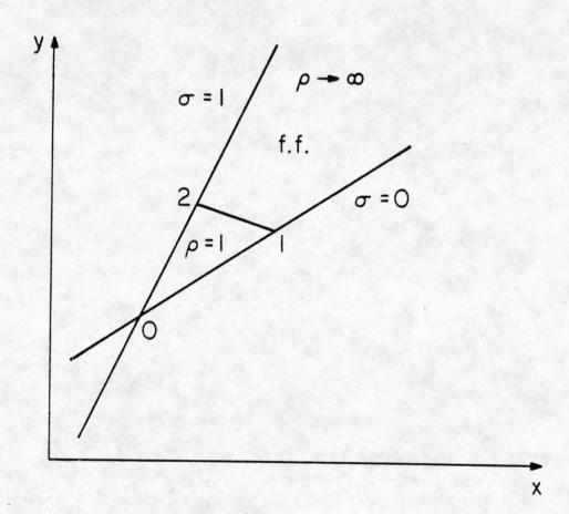
Figure 4b. Infinite element type II.
