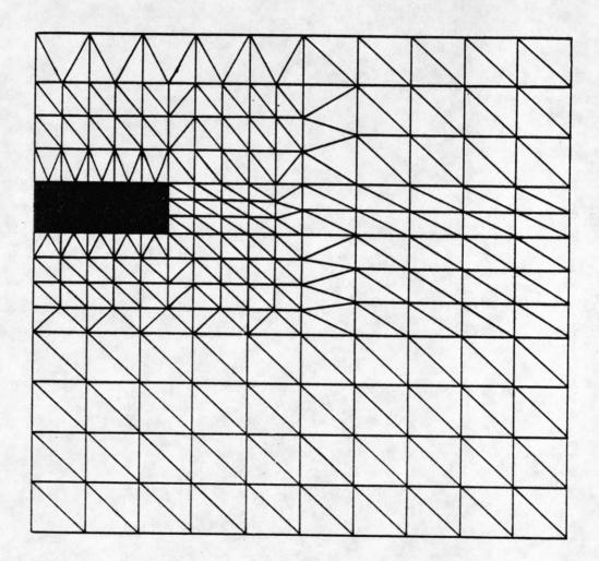
Figure 7. Triangular mesh for thick-strip transmission line with 153 nodes and 351 elements.
