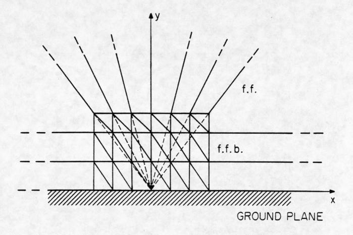
Figure 4a. Line consisting of a system of conductors placed above ground plane.
