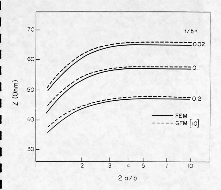
Figure 8. Characteristic impedance Z of thick-strip transmission line.
