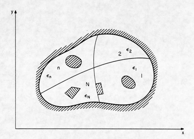
Figure 1. Cross section of a microwave transmission line.
