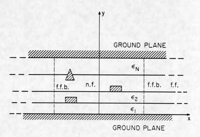
Figure 3a. Line consisting of a system of conductors placed between two ground planes.
