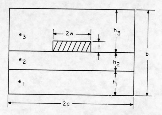
Figure 6. Thick-strip transmission line with multidielectric layers and shielding structure
