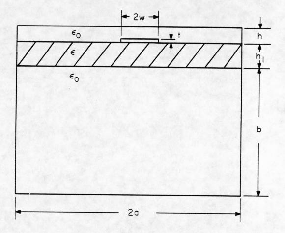
Figure 9. Generic cross-section of inverted microstrip with shielding structure
