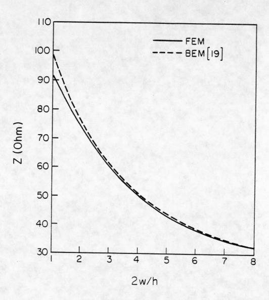
Figure 10. Characteristic impedance Z of shielded inverted microstrip line versus shape ratio 2w/h.
