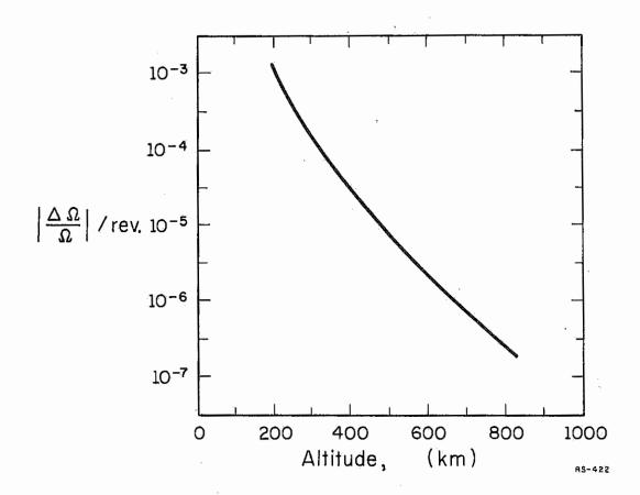
Figure 6.5. Relative average spin decay of a cone disk satellite per (circular) orbit.
