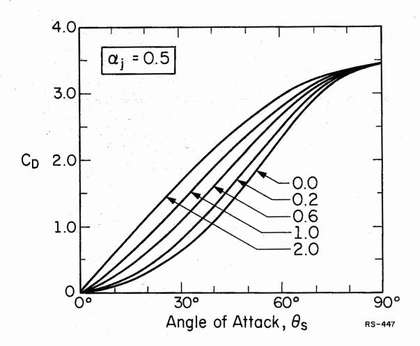
Figure 4.2. Drag coefficient of a non-spinning disk at angles of attack varying the generalized model parameter  $P_j$ .
