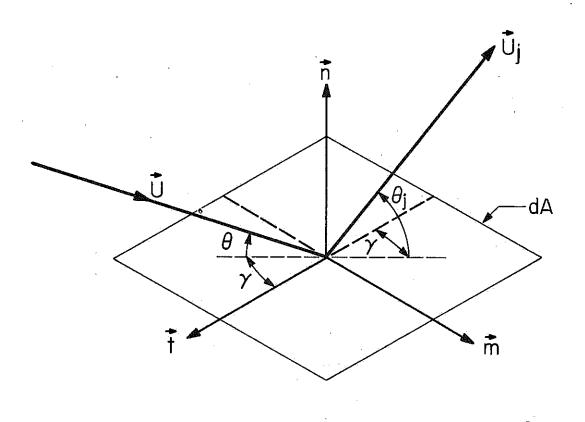
Figure 3.2. Local coordinate system on the surface element.
