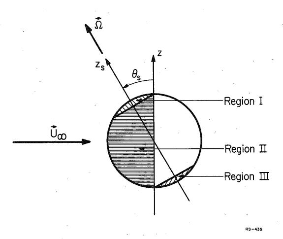
Figure 3.9. Regions of sphere surface exposed to the flow.
