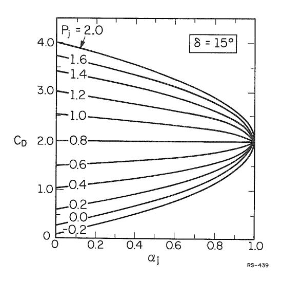
Figure 4.6. Drag coefficient of a non-spinning cone, with axis parallel to the flow, as a function of the generalized model parameters.
