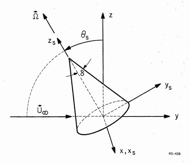
Figure 3.7. Spinning cone at angle of attack.
