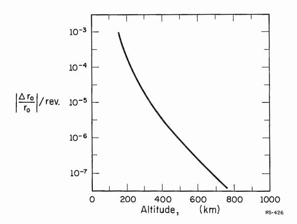
Figure 6.3. Relative average altitude loss per (circular) orbit for a cone-disk satellite.
