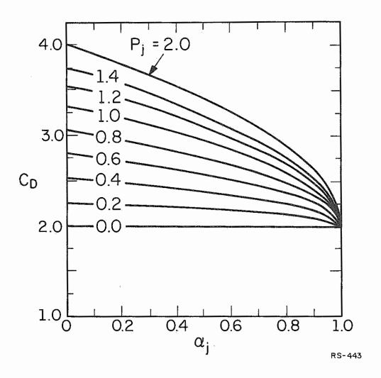
Figure 4.8. Drag coefficient of a non-spinning sphere as a function of the generalized model parameters.
