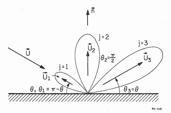
Figure 6.6. Notation for a possible three-lobed reflection.
