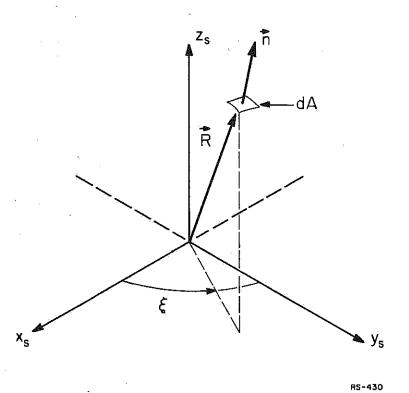
Figure 3.4. Orientation of surface element in the body coordinate system.
