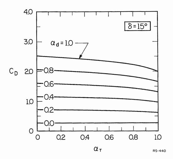
Figure 4.5. Drag coefficient of a non-spinning cone, with axis of the cone parallel to the flow, as a function of the Maxwell model parameters.
