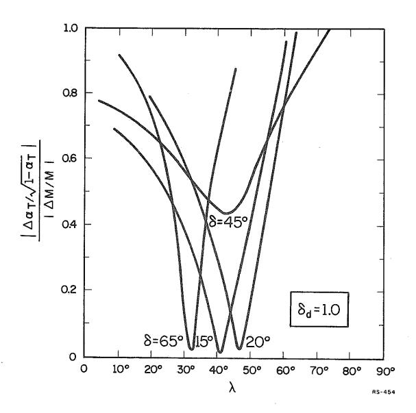
Figure 6.1. Maximum error in determining  $\sqrt{1-\alpha_T}$  using a cone-disk shaped satellite as a function of  $\lambda$  and  $\delta$ .
