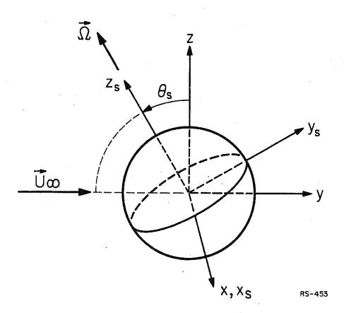
Figure 3.8. Spinning sphere at angle of attack.
