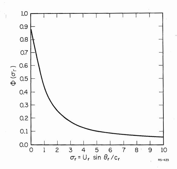
Figure 2.7. Plot of the coefficient of the normal component of force for the Nocilla model as a function of  $\sigma_{\bf r}$
