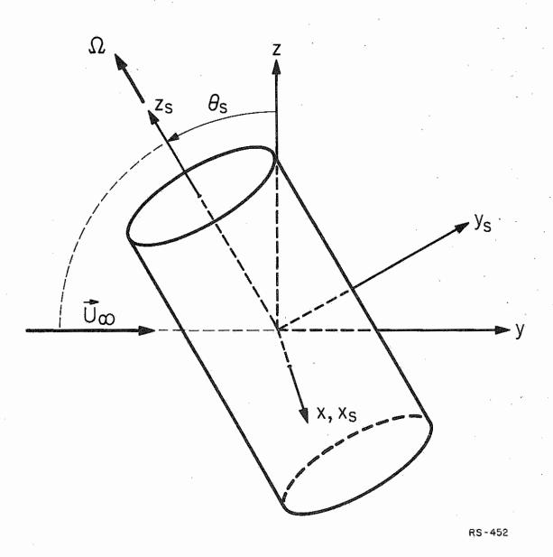
Figure 3.6. Spinning cylinder at angle of attack.
