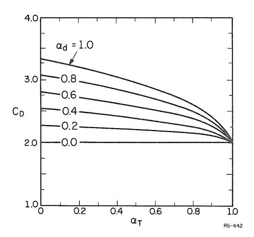
Figure 4.7. Drag coefficient of a non-spinning sphere as a function of the Maxwell model parameters.
