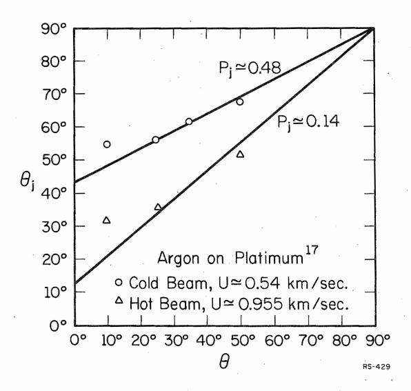
Figure 2.8. Comparison of experimental data <sup>17</sup> with the first approximation to an angle-of-reflection law of the generalized model.
