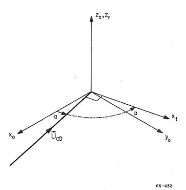
Figure 5.2. Coordinate system for force components.
