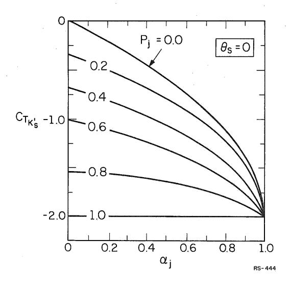
Figure 4.9. Coefficient of slow down torque on a spinning cylinder at zero angle of attack as a function of the generalized model parameters.
