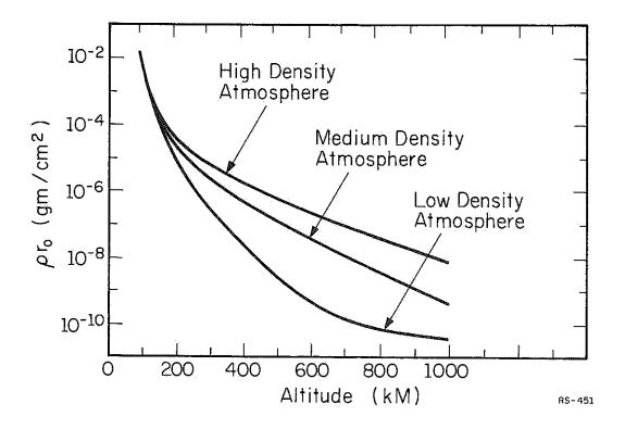
Figure 6.2. High, low, and medium atmospheric density variation with altitude (from tables in Reference 29).
