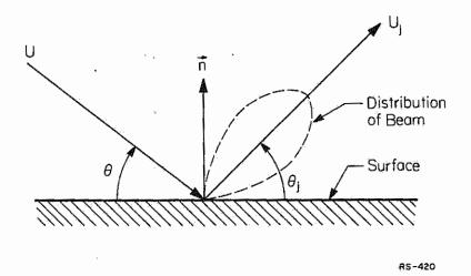
Figure 2.1. Notation used in the generalized model.
