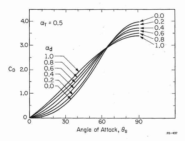
Figure 4.1. Drag coefficient of a non-spinning disk at angles of attack varying the Maxwell model parameter  $\alpha_{\rm d}$ .
