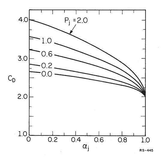
Figure 4.4. Drag coefficient of a non-spinning cylinder, with axis of cylinder perpendicular to the flow, as a function of the generalized model parameters.
