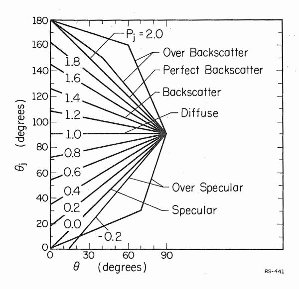
Figure 2.9. The full range of possible angle-of-reflection laws in the generalized model.
