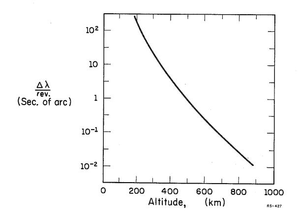
Figure 6.4. Relative average angular precession of spin-axis of a conedisk satellite per (circular) orbit.
