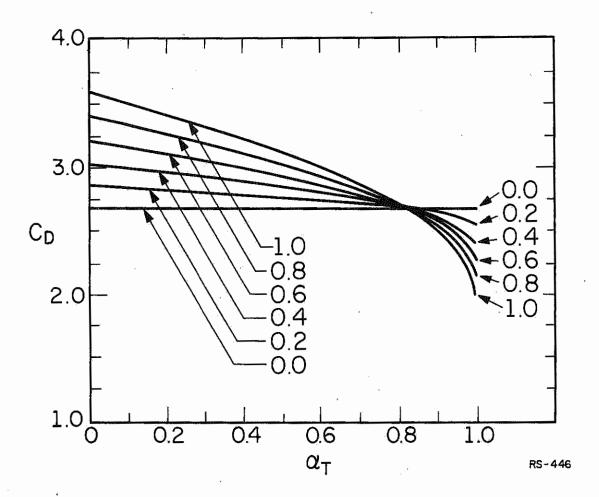
Figure 4.3. Drag coefficient of a non-spinning cylinder, with axis of cylinder perpendicular to the flow, as a function of the Maxwell model parameters.
