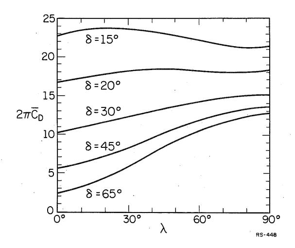
Figure 5.4. Average drag coefficient of a cone-disk shaped satellite as a function of  $\lambda$  and  $\delta$ .
