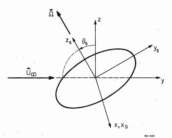
Figure 3.5. Spinning disk at angle of attack.
