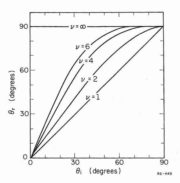
Figure 2.4. Plot of Schamberg's angle-of-reflection law.
