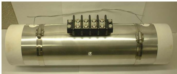
Figure 3.12 Cylindrical furnace for ultrasonic spray pyrolysis. Note that the picture is horizontally oriented. For syntheses, furnace was vertical. Photo Credit: Wong Suh.
