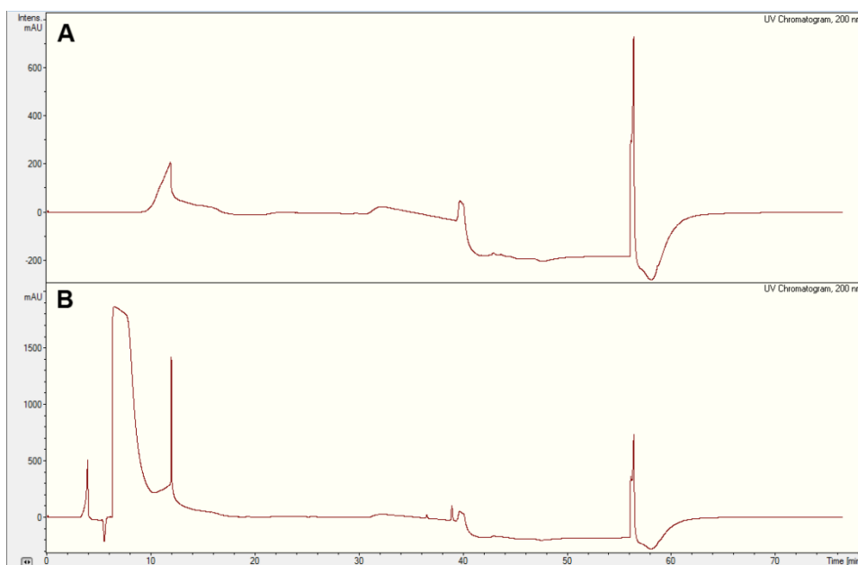
Figure 3.2. LC-MS UV chromatograms of a blank without any sample (A) and a BFC (NO 2 A-alkyne) sample (B). The same LC-MS method was used for all samples, and all samples had similar peaks from 0-12 min. The large peaks from ~6-12 min are due to a small amount of DMSO in samples.
