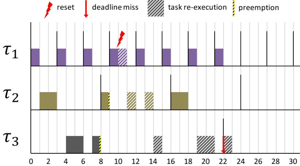
Figure 5.1: Example of fully preemptive system with 3 tasks \tau_1 = (1, 3) ; \tau_2 = (2, 8) ; \tau_3 = (4, 22) , and restart at t = 10 - \epsilon ( C_r = 0 ). The taskset is schedulable without restarts, however, restart and task re-execution causes a deadline miss at t = 22 .
