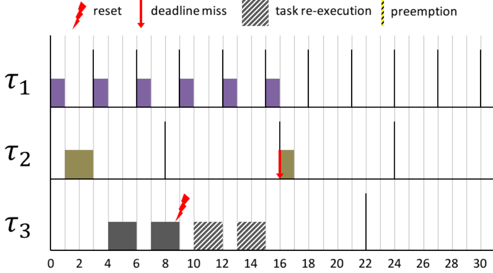
Figure 5.6: Example of system with 3 tasks \tau_1 = (1, 3) ; \tau_2 = (2, 8) ; \tau_3 = (4, 22) , where \tau_2 and \tau_3 have a preemption threshold of \lambda_2 = 1 and \lambda_3 = 2 , respectively. Restart occurs at t = 9 - \epsilon ( C_r = 0 ). The task set is not schedulable.
