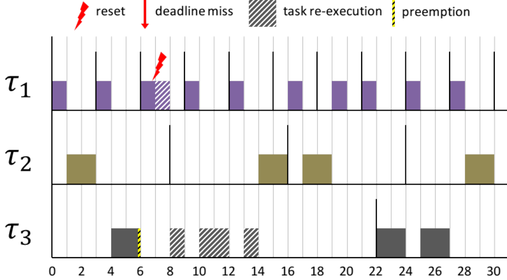
Figure 5.5: Example of system with 3 tasks \tau_1 = (1, 3) ; \tau_2 = (2, 8) ; \tau_3 = (4, 22) , where \tau_2 and \tau_3 have a preemption threshold of \lambda_2 = 1 and \lambda_3 = 2 , respectively. Restart occurs at t = 7 - \epsilon ( C_r = 0 ). In this case, the task set remains schedulable.
