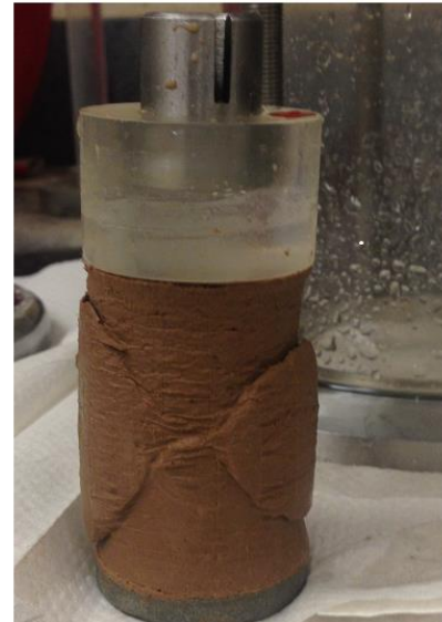
Figure 6.8. Photos of specimens at the end of consolidated undrained triaxial compression tests with porewater pressure measurement (a) budging in a Glen Forest Clay specimen consolidated at 5psi (b) single shear plane in a Beaumont Clay specimen consolidated at 80 psi (c) one distinct shear plane, and one shear plane not fully developed in a Brenna Clay specimen consolidated at 40 psi (d) two intersecting shear planes in Newmont Gold Quarry Clay specimen consolidated at 50 psi (1 psi = 6.89 kPa)
