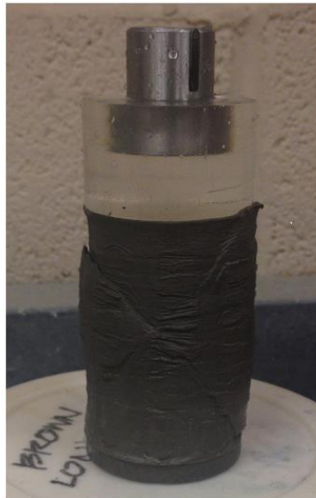
Figure 6.8. Photos of specimens at the end of consolidated undrained triaxial compression tests with porewater pressure measurement (a) budging in a Glen Forest Clay specimen consolidated at 5psi (b) single shear plane in a Beaumont Clay specimen consolidated at 80 psi (c) one distinct shear plane, and one shear plane not fully developed in a Brenna Clay specimen consolidated at 40 psi (d) two intersecting shear planes in Newmont Gold Quarry Clay specimen consolidated at 50 psi (1 psi = 6.89 kPa)
