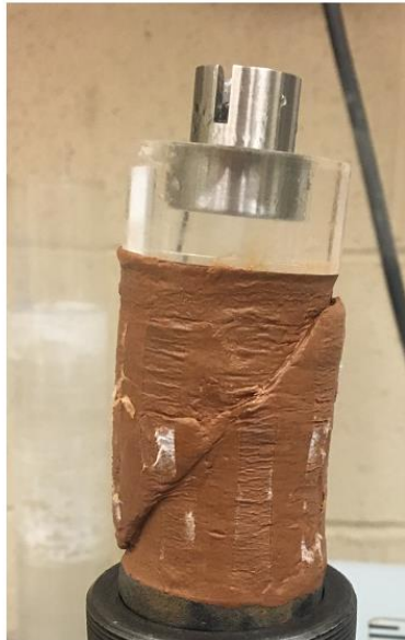
Figure 6.9. Photos of specimens at the end of consolidated drained triaxial compression tests (a) cylindrical shape of a Brenna Clay specimen consolidated at 10psi (b) budging in a Kuykendahl Clay specimen consolidated at 30 psi (c) single shear plane in a Mud Gully Clay specimen consolidated at 30 psi (d) single shear plane in a Brenna-Sodium Montmorillonite mixture 1 specimen consolidated at 80 psi (1 psi = 6.89 kPa)
