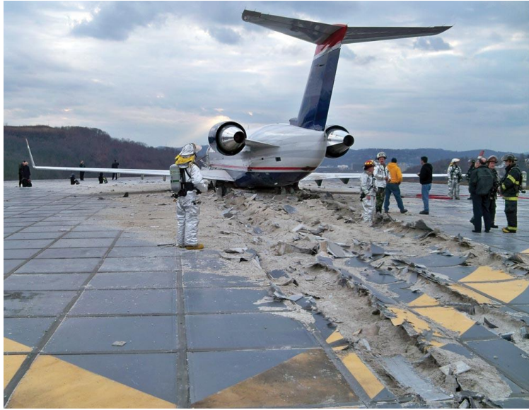
Figure 5.11. An aircraft stopped by EMAS [11].
