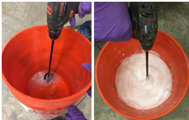
Figure 1.7. Preparation of the aqueous foam in a bucket with a hand mixer: (left) before and (right) after the mixing.
