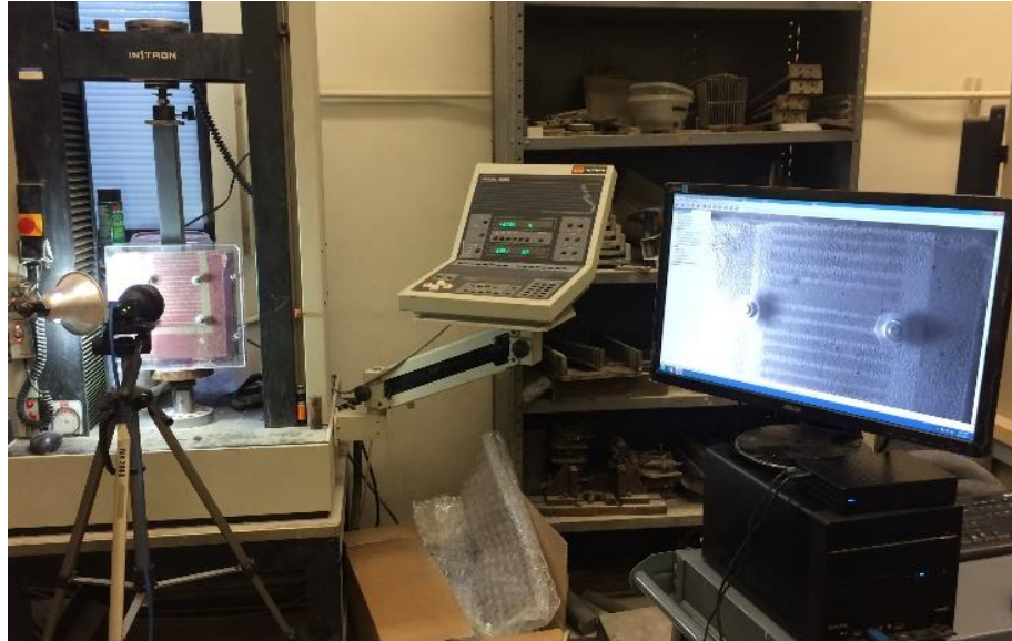
Figure 4.14. Test setup used for the DIC analysis.
