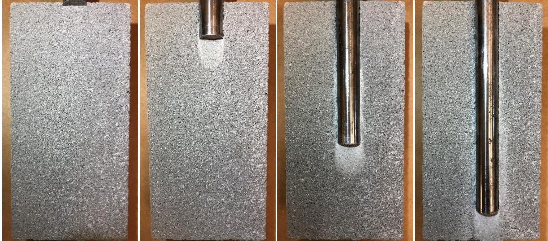
Figure 3.3. Development of the local densification on the same cross-section of a C 0.6 cylinder specimen. The crushing depths were 1, 30, 120, and 180 mm, corresponding to the elastic, transitional, plateau phase, and densification crushing phases, respectively. The densified region is distinctive from the uncrushed foam.
