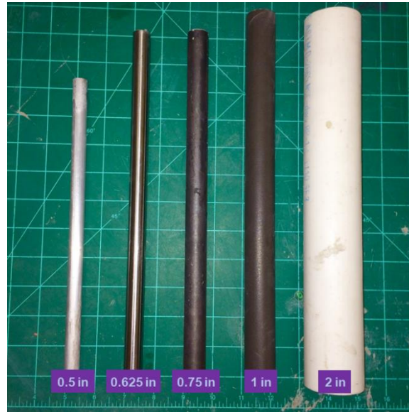
Figure 4.3. Indenters with different diameters used in the penetration test.
