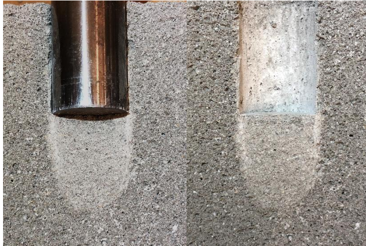
Figure 3.5. Magnified view of the local densification of the C_0.6 specimen cross-section, before and after removing the indenter.
