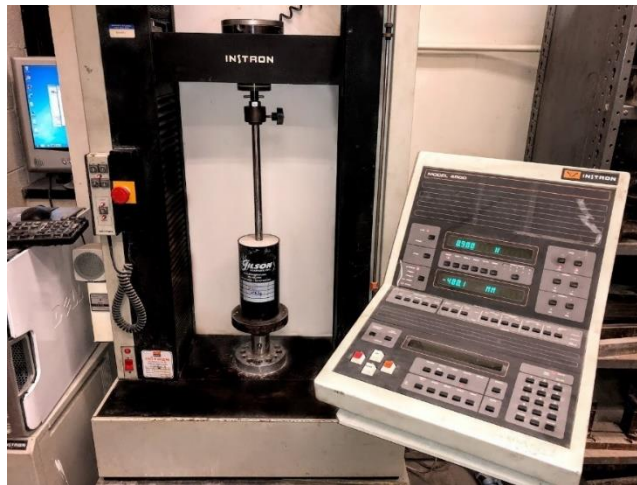
Figure 3.1. Testing setup for the penetration test. The Instron 4052 loading frame is coupled with a 10 kN load cell.
