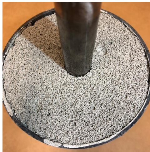
Figure 3.4. Top surface of a C 0.6 cylinder specimen after the test, in which no crack was seen.
