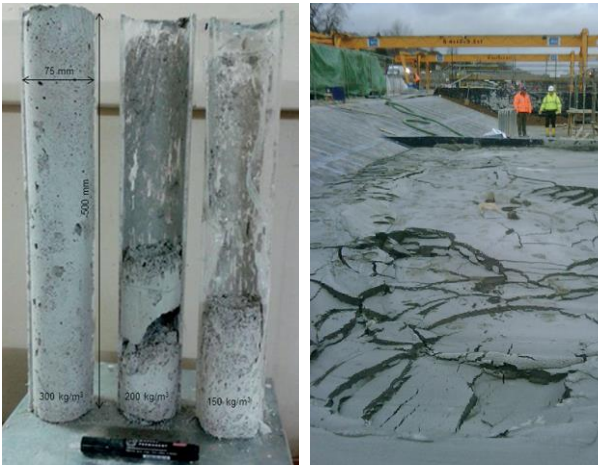
Figure 1.4. Examples of the instability of foam concrete due to collapse at early ages: (left) in the lab and (right) in the field [22].
