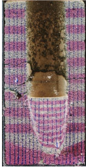
Figure 4.2. A sample ( 0.4 \text{ g/cm}^3 ) showing horizontal and Lateral deformation of the densification.
