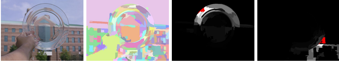
Figure 4.5: From left to right: a test image, its initial segmentation based on color and texture, two selected regions (red) and the affinity values of all other regions. Brighter intensities indicate higher values.
