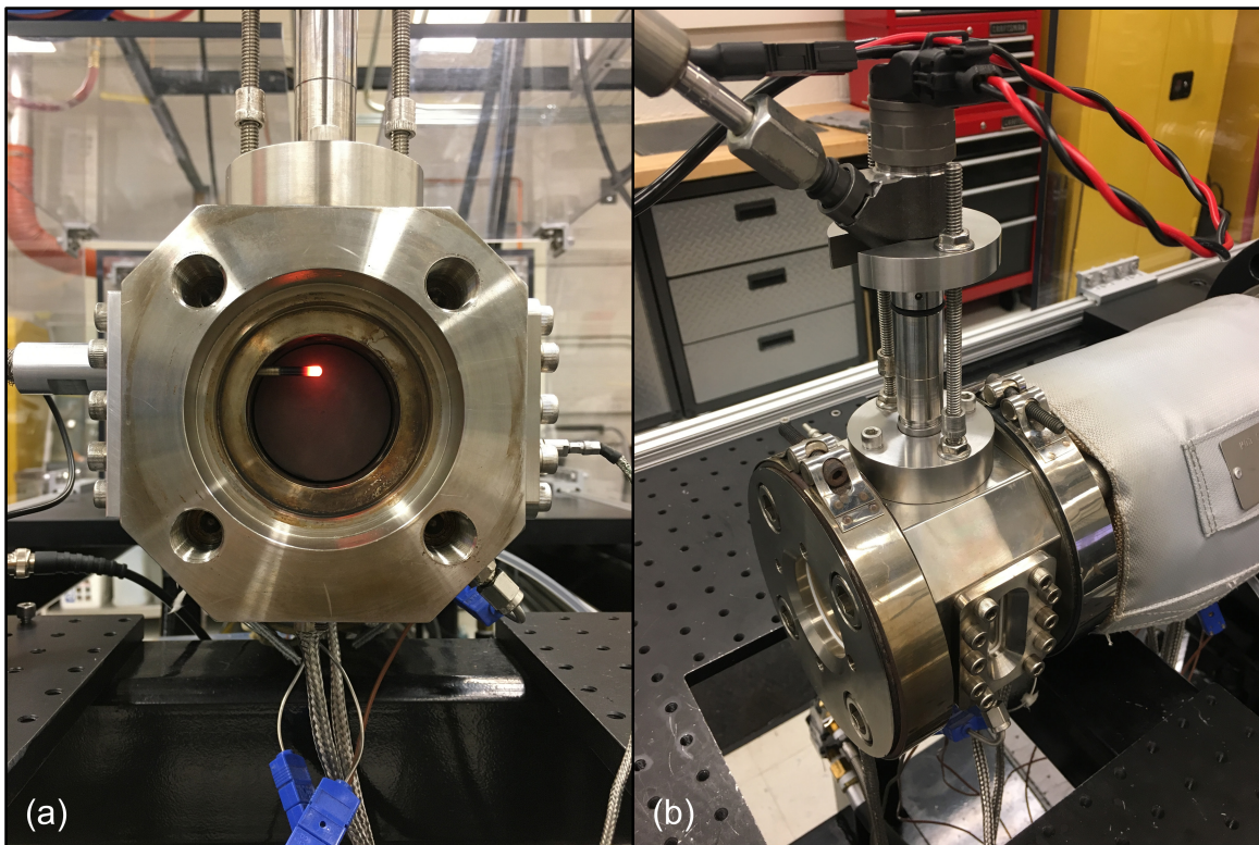
Figure 5. Activated ignition device in rapid compression machine combustion chamber (a) and mounted injector (b)
