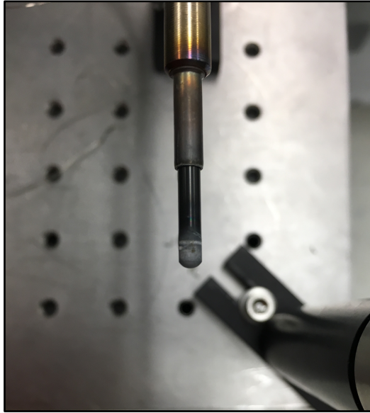
Figure 30. Oxidation of operational ceramic heating element after 2 weeks for 10 V benchtop durability experiment
