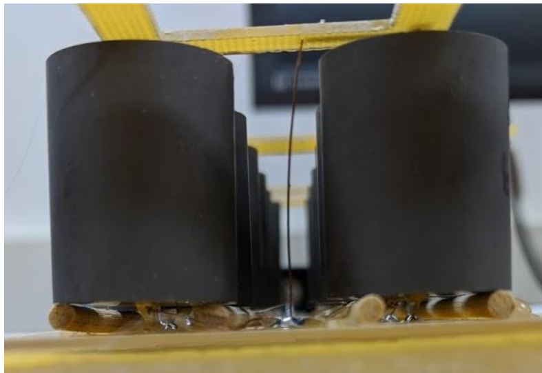
Fig. C.4. Rod PADA array elements mounted on wooden slates to ensure vertical alignment.
