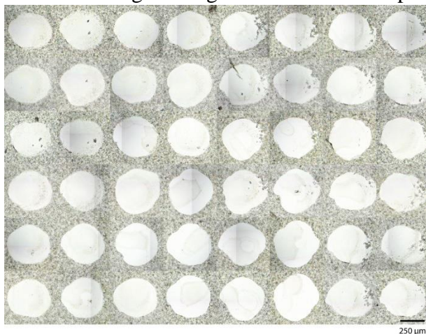
Figure 4.7. Montage of extraction areas. Each spot is the result of a 5 s extraction time from a DHB-coated microscope slide. The extraction profile is roughly circular, with an average radius of 206.3 \pm 1.7 \mu\text{m} .
