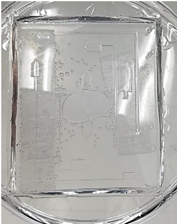
Figure 10.5. 3D models and 3D-printed channel molds for top and bottom layers of the device.
