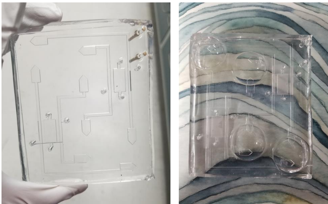
Figure 10.6. Fabricated devices without marble wells ( left ) and with marble wells ( right ).
