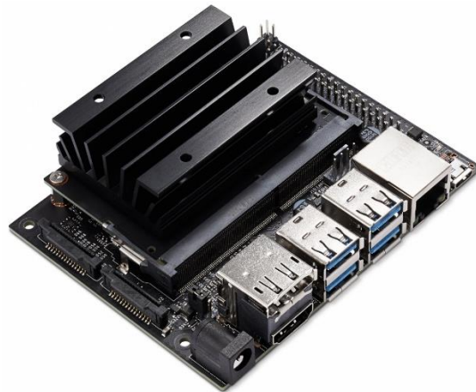
Figure 69 Jetson Nano small AI computer developed by NVIDIA[229]
