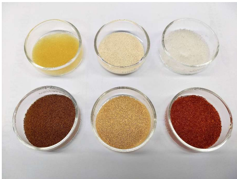
Fig. 2.1. Photo of anion exchange resins. First row (left to right): HPR9200; HPR9600; and IRA67. Second row (left to right): hybrid HPR9200; hybrid HPR9600; and hybrid IRA67.
