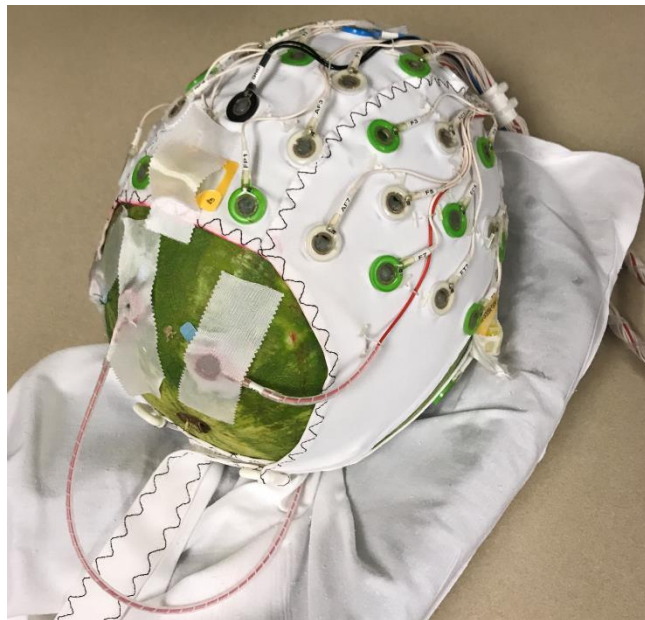
Figure 1: Watermelon ‘phantom’ outfitted with the 64-channel BrainProducts EEG cap.
