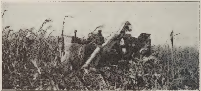
FIG. 2.—TWO-ROW HUSKERS OPERATE WITH LESS MAN LABOR AND POWER COST PER ACRE THAN ONE-ROW MACHINES
