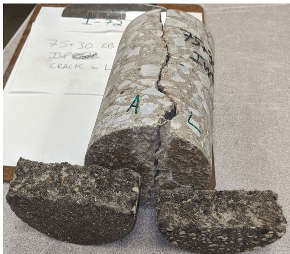
C. 75+30 EB IWP longitudinal crack on leave; stripping on leave only
