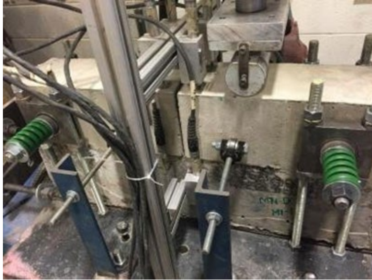
C. Composite beam setup with HMA interlayer
