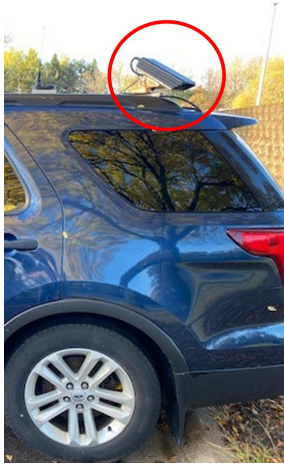
(a) Mobile RWIS mounted on supervisor vehicle
