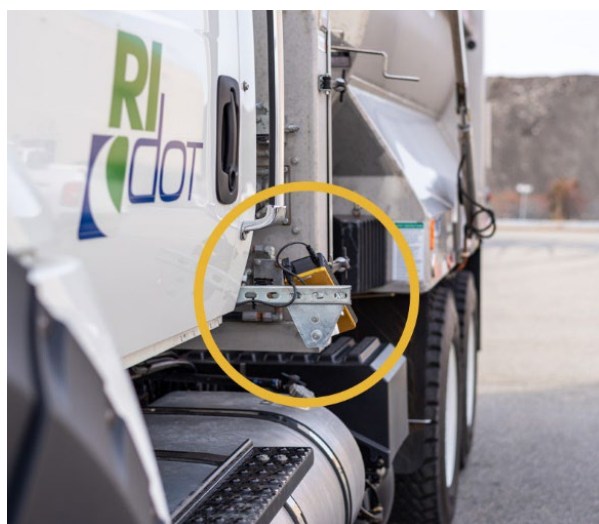
(b) Mounting RWIS unit along wheelhouse
