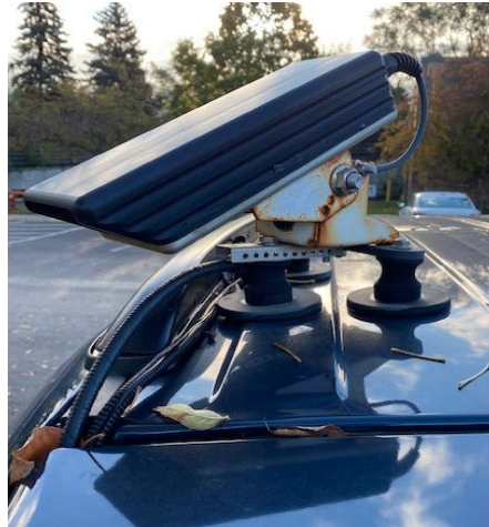
(b) Close up of magnetic mount on supervisor vehicle
