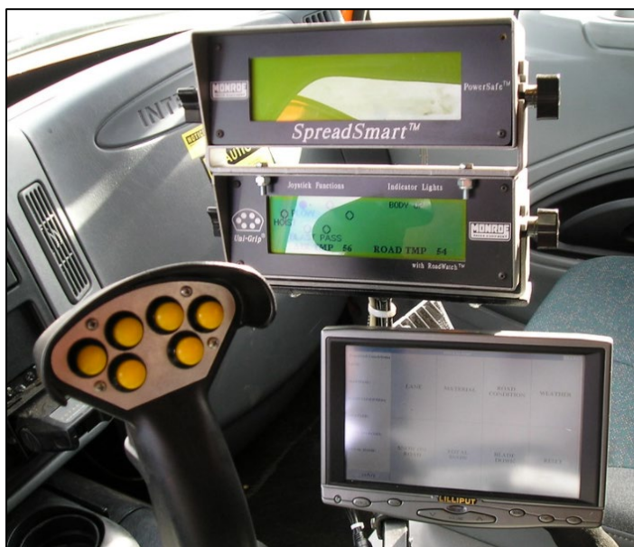
Figure 6. Photo. CDOT snowplows equipped with mobile RWIS and MDSS display (CDOT 2013).
