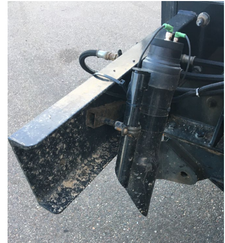
(c) Mobile RWIS mounted on front bumper of snowplow
