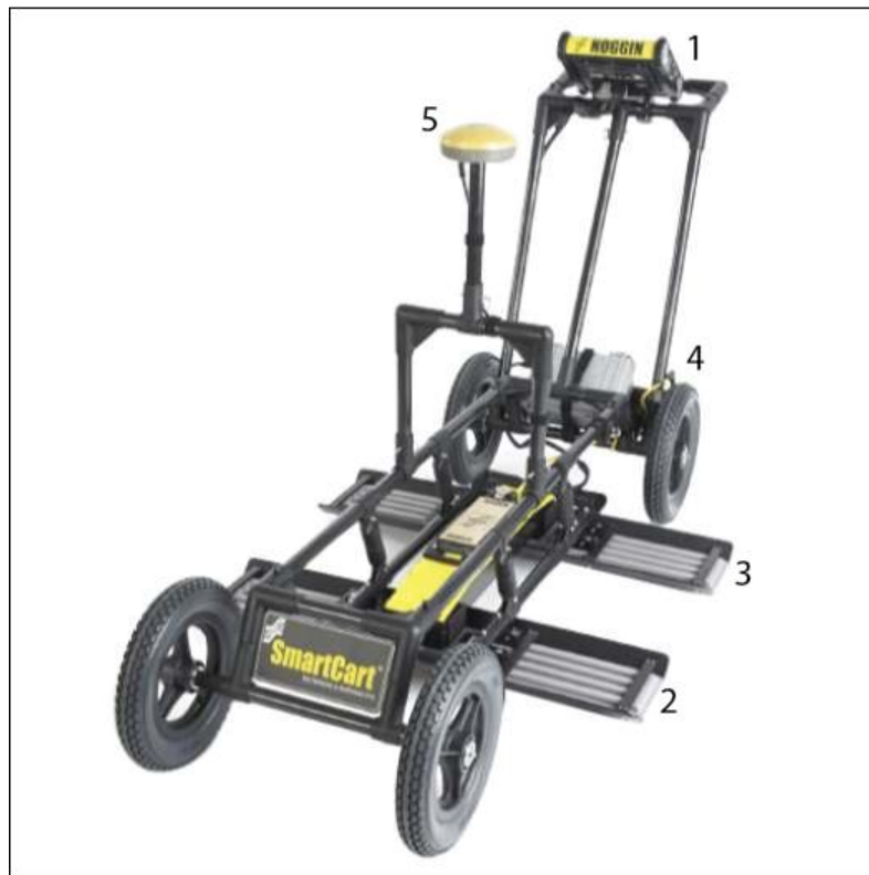
Figure 2.11: Basic GPR setup: 1) controller; 2) transmitter; 3) receiver; 4) Encoder wheel for measuring distance; 5) GPS. Edited Image from Sensors and Software (2021).
