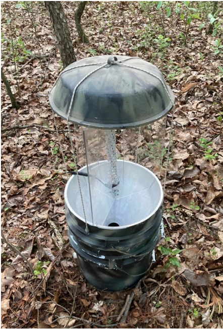
Figure 1. A bucket trap in the field at Sand Ridge State Forest. The battery and timer controlling the LEDs are behind the trap in this image.
