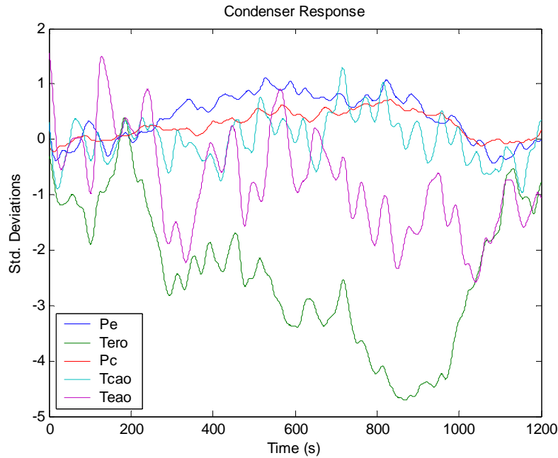
Figure 6.21 - Output deviation in the input-output response of the system to valve excitation when a 10% decrease in air flow has occurred in the condenser
