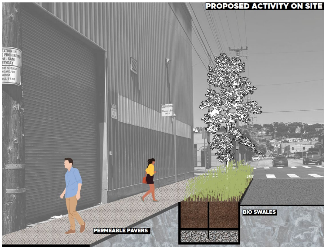
Fig 7.14: A perspective of how pavements with introduction of bioswales and urban farms can look.
